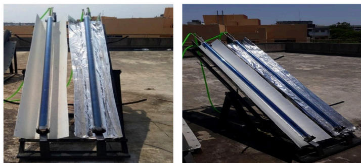
Figure 2. Schematic diagram of hybrid solar desalination system (ETC + CPC)
