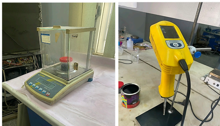
Figure 5. Nanotube painting preparation devices
