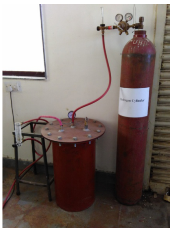
Figure 6. Hydrogen fuel supply setup with flame trap
