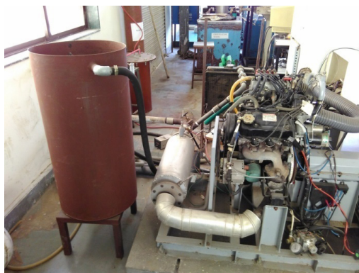
Figure 7. HCNG setup with engine cooling system
