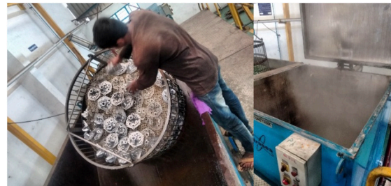
Figure 5. Photo of hot water curing tank in CMI plant
