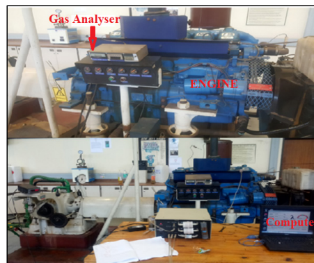
Figure 4. Experimental setup of marine diesel engine [38] permissions from Ain Shams Engineering Journal
