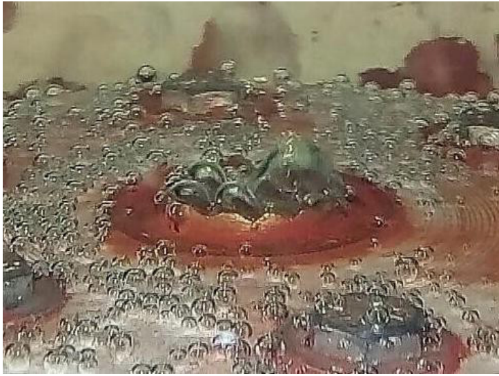
Figure 12. Boiling phenomena on a v-structured surface
