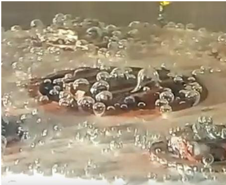
Figure 13. Boiling phenomena on a square-structured surface
