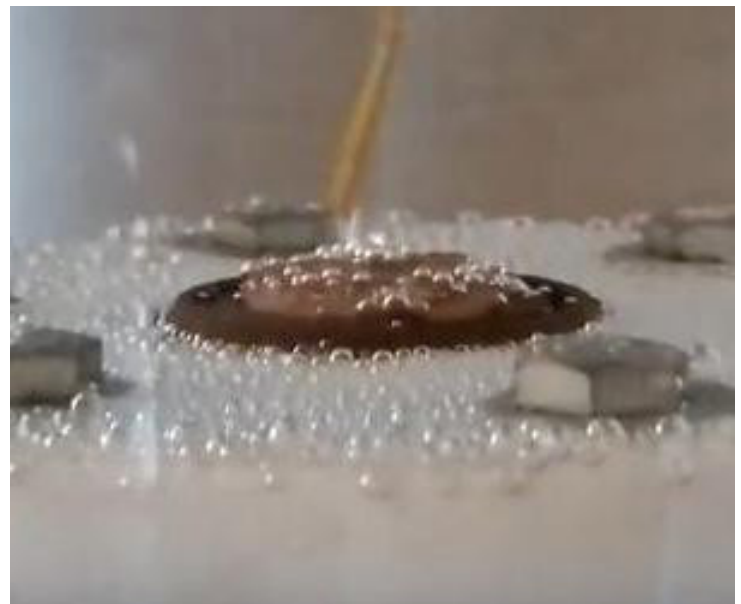
Figure 11. Boiling phenomena on a plain surface
