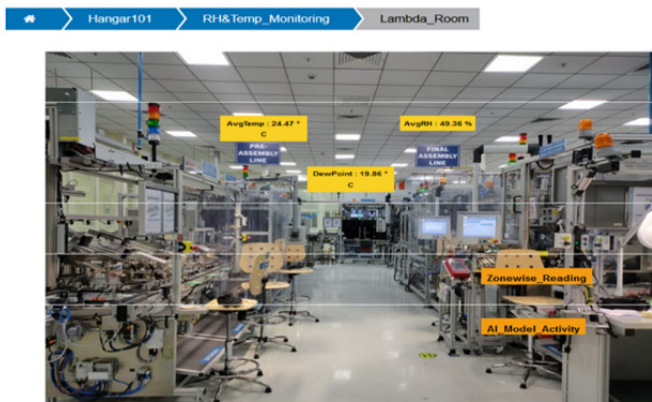
Figure 14. Controlled temperature & humidity & within the clean-room range
