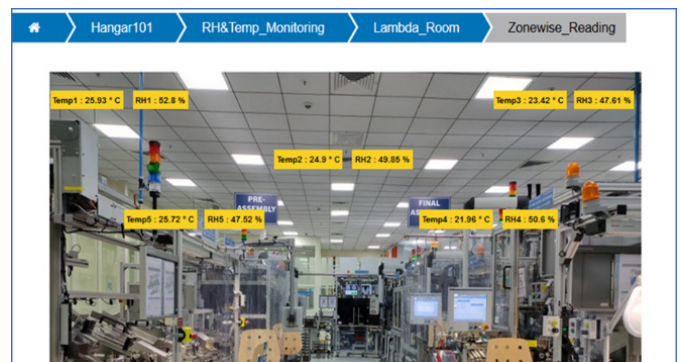
Figure 3. Internal Bosch Online monitoring system showing the RH and Temperature values
