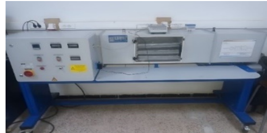
Figure 9. Convective dryer CE 130 The air flow was set at 2.5 m3 and the temperature was set at 40 C°
