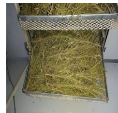
Figure 9. Convective dryer CE 130 The air flow was set at 2.5 m3 and the temperature was set at 40 C°
