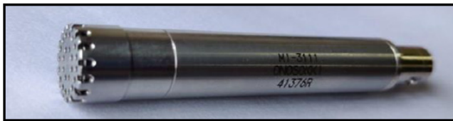
Figure 6. Onosokki microphone Mi-1433 with preamplifier Mi-3111 used for acoustic measurements
