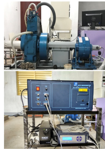
Figure 3. Tested engine, smoke meter and exhaust gas analyzer
