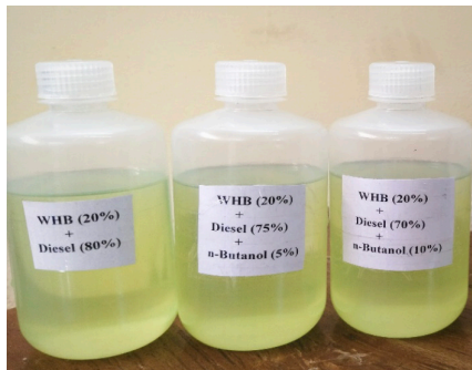
Figure 4. Blended mixtures of WHB20D80, WHB20D75B5, and WHB20D70B10
