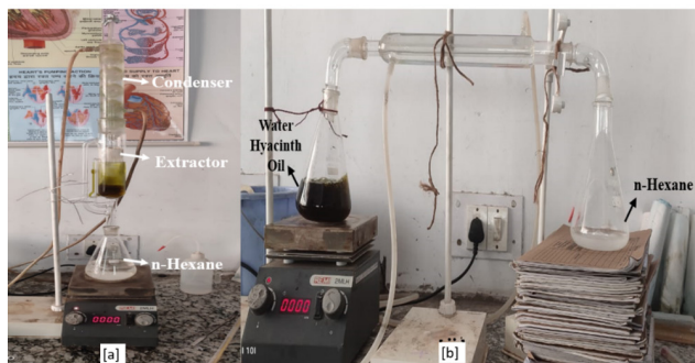
Figure 2. Extraction of oil (a) Soxhlet apparatus (b) Distillation unit
