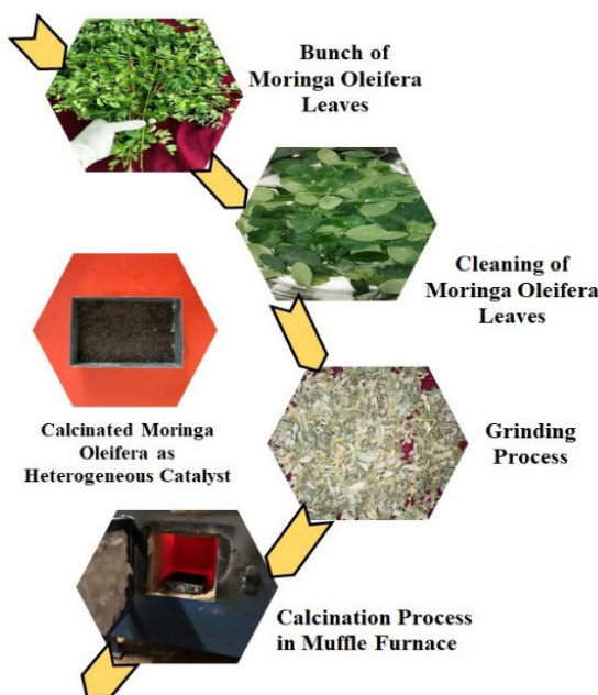
Figure 6. Step-by-step preparation of the moringa oleifera leaves as a heterogeneous catalyst
