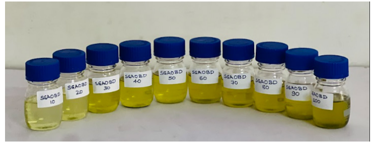
Figure 8. The blending of sea green algae oil biodiesel with diesel
