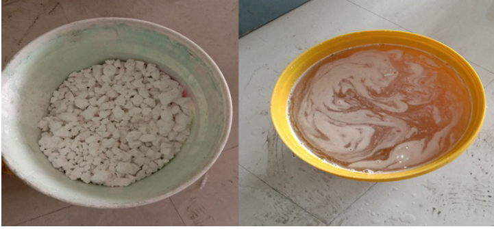
Figure 4. Liquid calcium chloride desiccant solution employed in the absorption and regeneration processes
