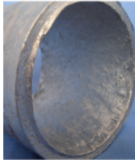
Figure 5. (b) Cast cylinder with Asbestos Insulation.
