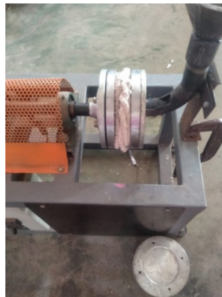
Figure 4. (b) Mould with Asbestos Insulation.
