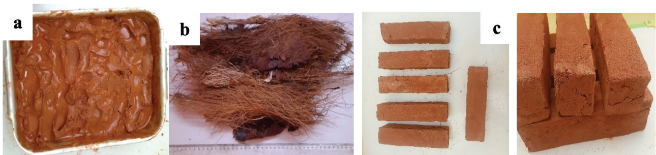
Figure 3. sample preparation a: adobe, b: palm fiber, c: samples [photo by author].
