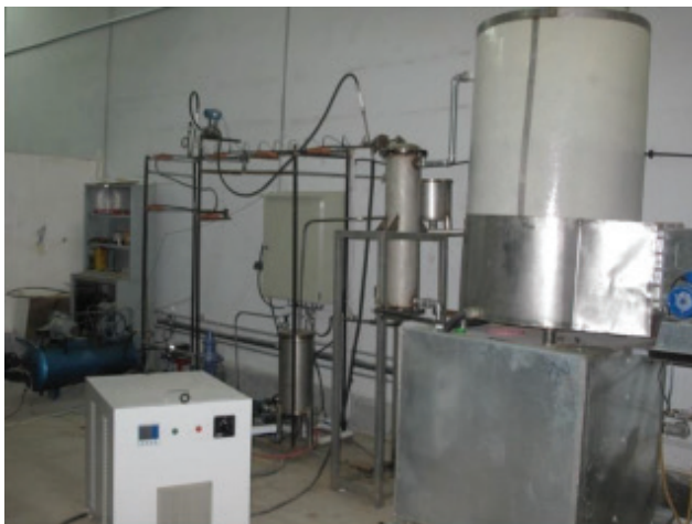
Figure 7. Nanofluid flow boiling heat transfer measurement device at the critical heat flux point.
