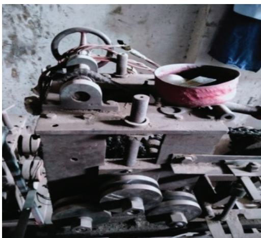
Figure 8. Bending Machine used for Parabolic Shape.
