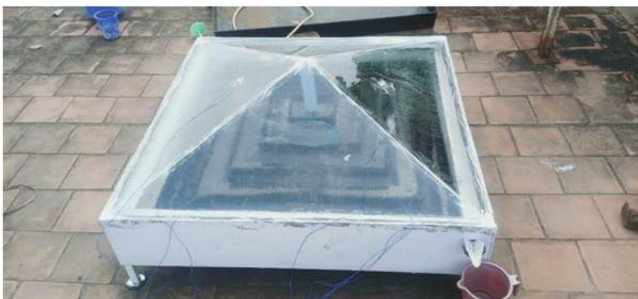
Figure 1. Pyramid shaped solar still with fins attached.
