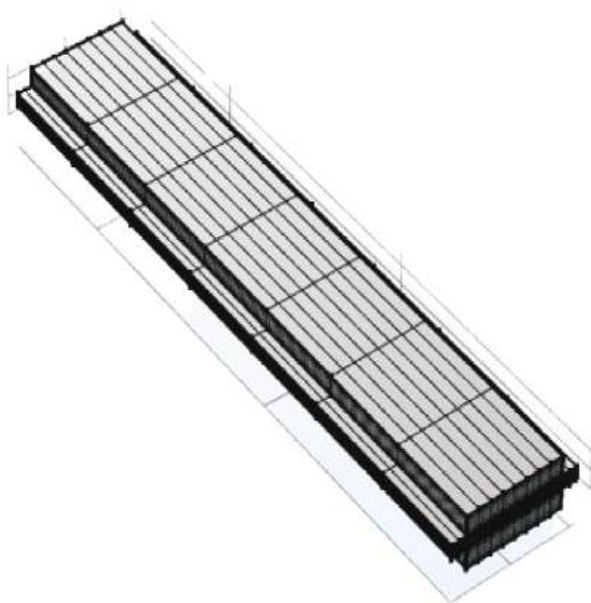
Figure 2. Meshed image of the modeled fuel cell.
