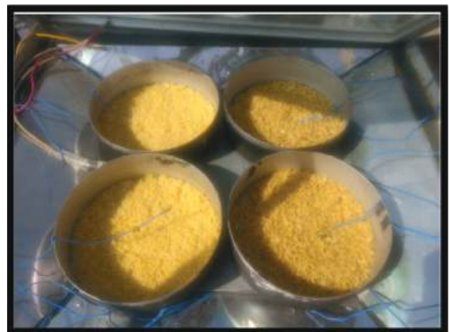
Figure 10. Toor daal and Moong daal placed in the hybrid solar cooker for cooking during experimentation.
