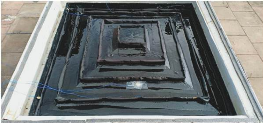
Figure 2. Pyramid shaped solar still with fins covered by black cloth.
