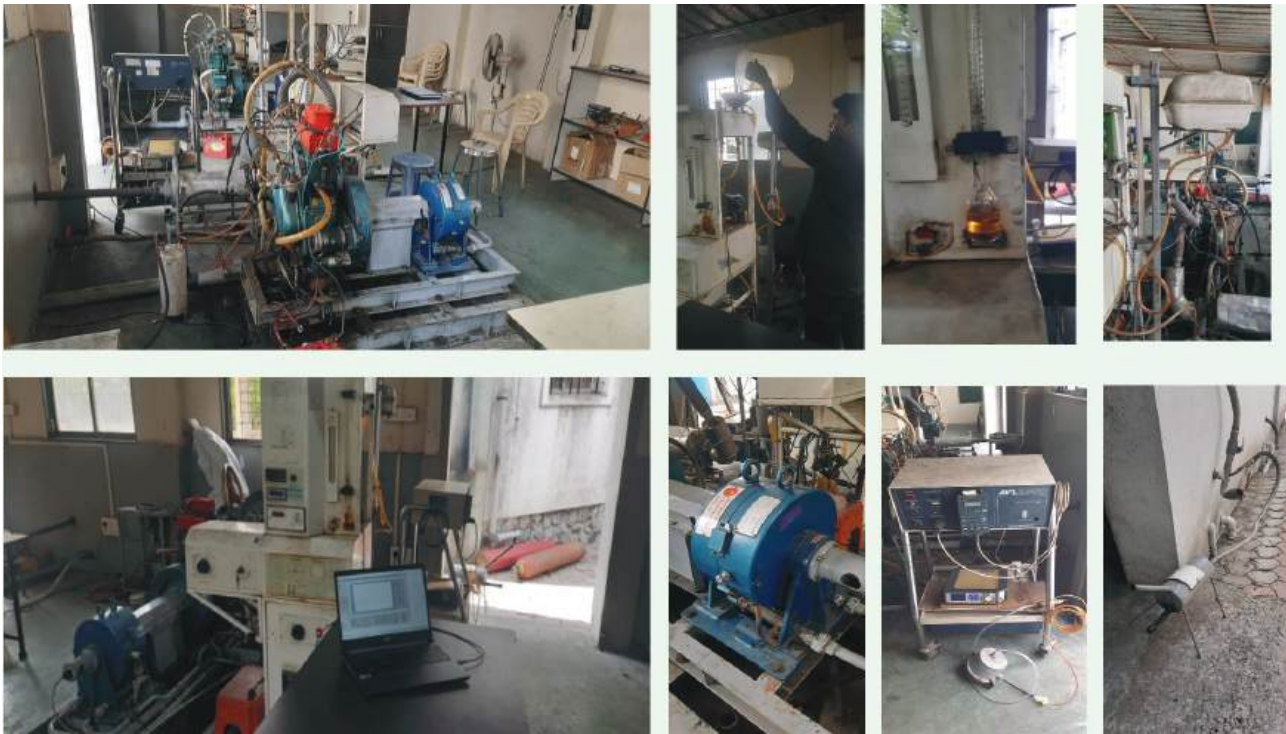
Figure 4. Variable compression engine experimental setup (Engine, Flue inlet system, flow measurement, control system, dynamometer, and Exhaust gas analyser system).
