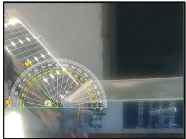
Figure 9. Photographic view of Hybrid solar cooker showing the inclination of photovoltaic panel with the horizontal plane.
