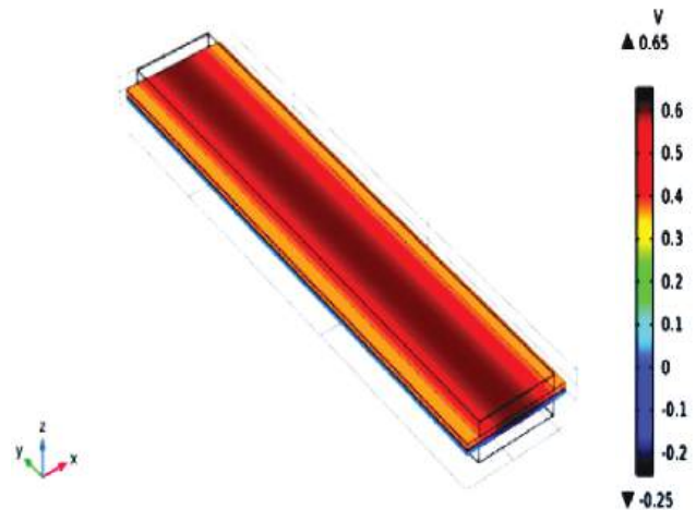
Figure 6. Contours of electrode potential of the fuel cell.
