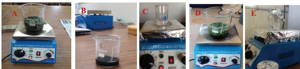
Figure 2. Shows prepared nanofluids of (A) CuO, (B) SiO 2 , (C) GO, (D) rGO, (E) Al 2 O 3 .
