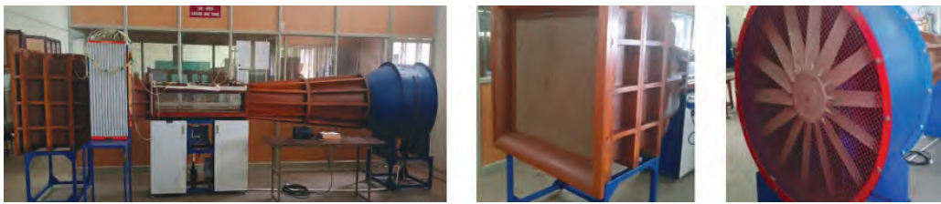
Figure 3. Low-speed subsonic wind tunnel facility
