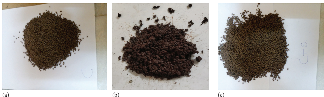
Figure 1. Photographs of heat treated (a) clay (b) clay-horse dung and (c) clay-sawdust desiccants.
