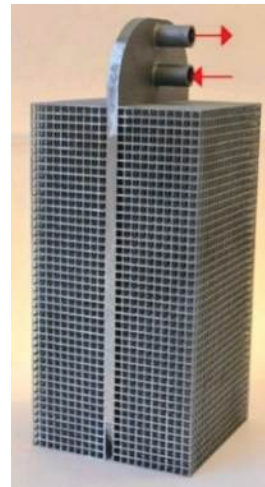
Figure 74. Lightweight HX design for thermal storage system. [From Yazdani et al. [134], with permission from Elsevier.]
