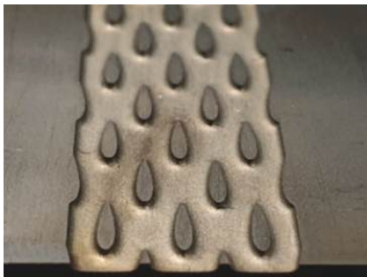
Figure 58. Optimized geometric configuration of airfoil fin in the PCHE. [From Park et al. [115], with permission from Elsevier.]
