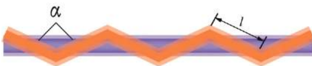
Figure 53. Geometric configuration of 120° angle combined channel PCHE. [From Liu et al. [109], with permission from Elsevier.]
