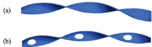
Figure 24. (a) Imperforated and (b) perforated twisted tape insert. [From Farhadi et al. [68], with permission from Elsevier.]
