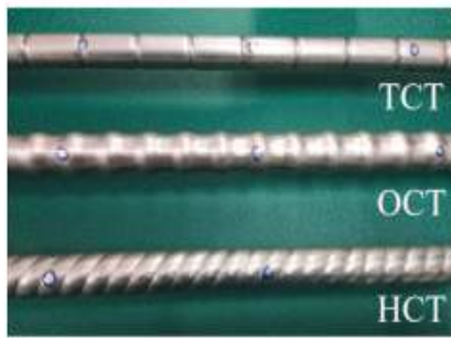
Figure 3. Geometrical models of a transversely corrugated tube (TCT), outward corrugated tube (OCT), and helically corrugated tube (HCT). [From Hu et al. [42], with permission from Elsevier.]
