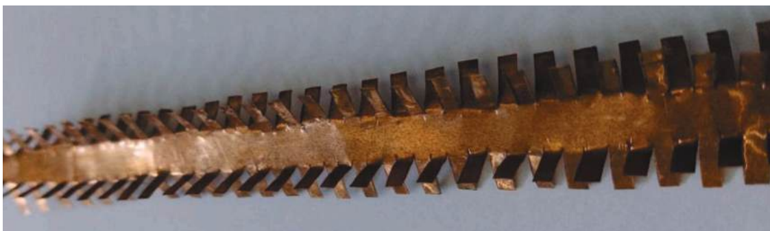
Figure 13. Square-cut copper VGs with a fin width of 2.5 mm. [From Hassan et al. [56], with permission from Elsevier.]
