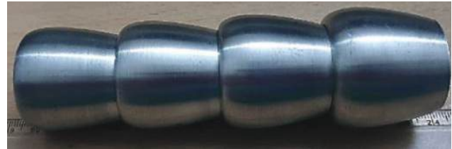
Figure 18. Airfoil-shaped turbulator with varying thickness profiles. [From Mousavi et al. [62], with permission from Elsevier.]
