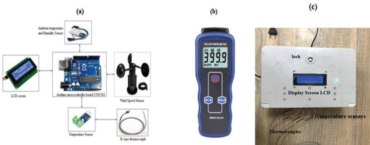
Figure 6. Measuring devices: a) Component Arduino b) Solar power meter c) Arduino device.
