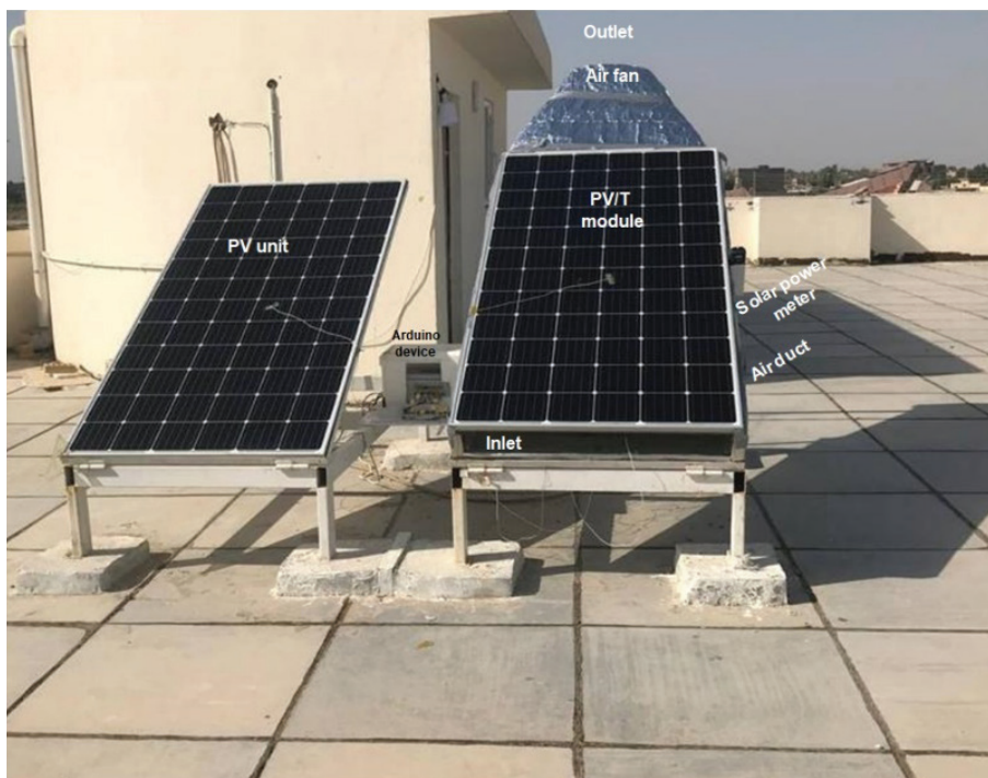
Figure 7. Experimental setup of the PV unit and PV/T system.
