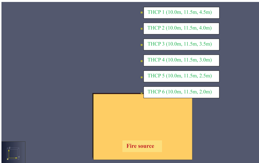
Figure 12. Arrangement of thermocouples.
