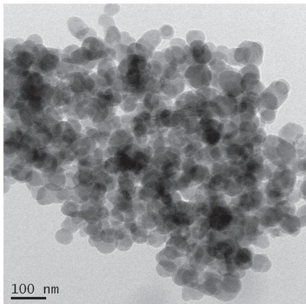
**Figure 1.** HRTEM pictograph of Al<sub>2</sub>O<sub>3</sub> nanoparticles.
