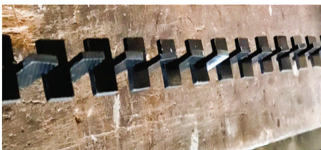
Figure 3. Continuous insert at 90° twist angle.
