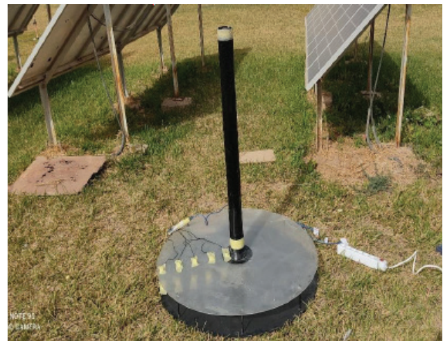
Figure 1. The solar chimney prototype.
