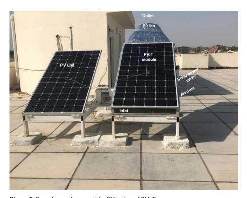
**Figure 7.** Experimental setup of the PV unit and PV/T system.
