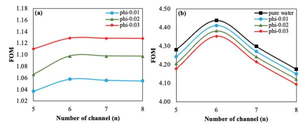
**Figure 27.** Variation of the FOM with channel counts for (a) Q=0.05046 lpm, (b) Q=0.05046 lpm,  $\epsilon$ =0.75.
