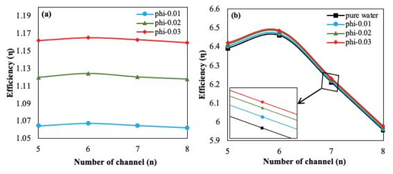
**Figure 24.** Variation of the heat transfer efficiency with channel counts for (a) Q=0.05046 lpm, (b) Q=0.05046 lpm,  $\epsilon$ =0.75.
