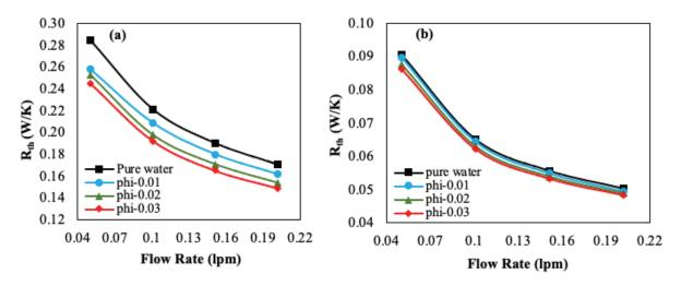
**Figure 12.** Variation of the thermal resistance with flow rate for n=05 (a) clear channel (b) porous channel at  $\epsilon$ =0.75.
