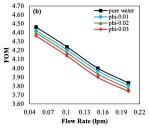
**Figure 25.** Variation of the FOM with flow rate for n=05 (a) clear channel (b) porous channel at  $\epsilon=0.75$ .
