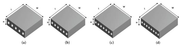
Figure 2. Heat sink schematic diagram at various channel counts (a) 5, (b) 6, (c) 7, (d) 8 respectively.
