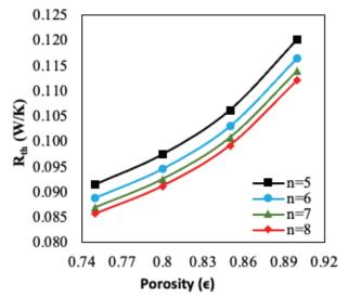
**Figure 16.** Variation of the thermal resistance with porosity at Q=0.05046 lpm, phi-0.01.
