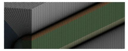
**Figure 3.** Represents the grid's distribution in the solid and fluid regions of the heat sinks.
