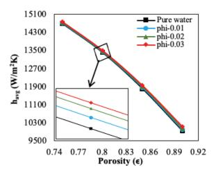
**Figure 8.** Variation of the average heat transfer coefficient with porosity for n=05 at Q=0.05046 lpm.
