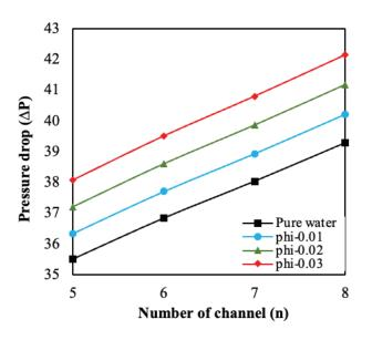
**Figure 20.** Variation of the pressure drop with channel counts (Porous) at Q=0.05046 lpm,  $\epsilon$ =0.75.
