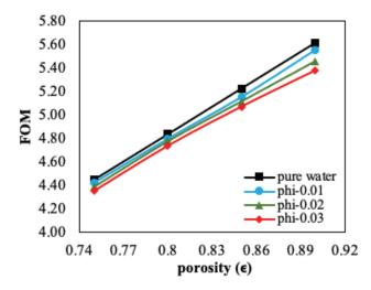
**Figure 26.** variation of the FOM with porosity for n=05 at Q=0.05046 lpm.
