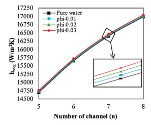
**Figure 10.** Variation of the average heat transfer coefficient with channel counts (Porous) at Q=0.05046 lpm,  $\epsilon$  =0.75.
