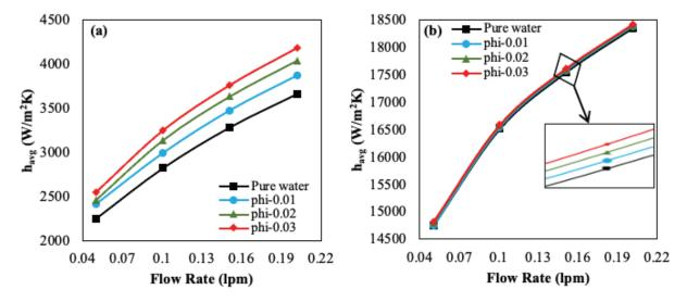
**Figure 7.** Variation of the average heat transfer coefficient with flow rate for n=05 (a) non-porous channel (b) porous channel at  $\epsilon = 0.75$ .
