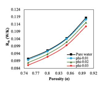
**Figure 13.** Variation of the thermal resistance with porosity for n=05 at Q=0.05046 lpm.
