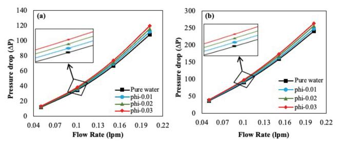
**Figure 17.** Variation of the pressure drop with flow rate for n=05 (a) clear channel (b) porous channel at  $\epsilon$ =0.75.
