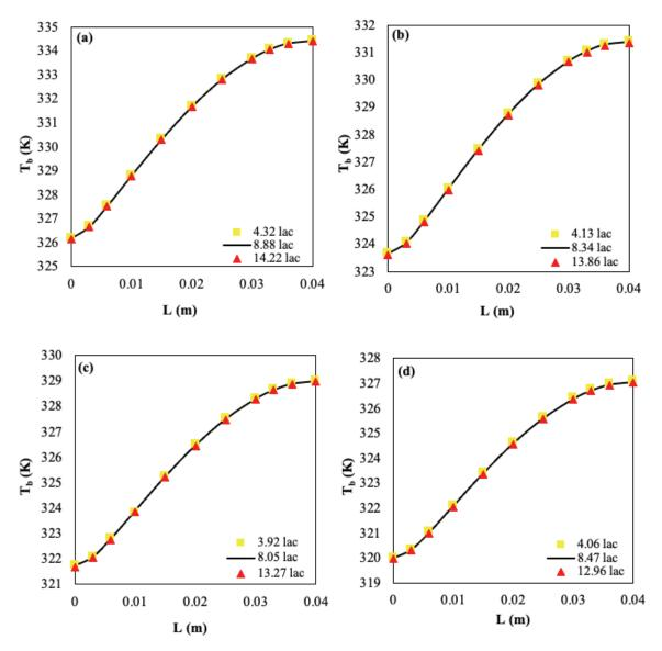
Figure 4. Grid independency test at various channel counts (a) n=05 (b) n=06 (c) n=07 (d) n=08 respectively.
