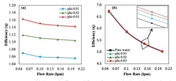
**Figure 22.** Variation of the heat transfer efficiency with flow rate for n=05 (a) clear channel (b) porous channel at  $\epsilon$ =0.75.
