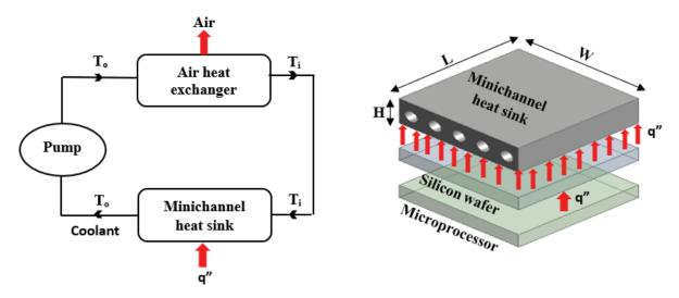
Figure 1. Schematic and working of minichannel heat sink in electronic cooling.
