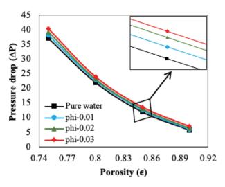
**Figure 18.** Variation of the pressure drop with porosity for n=0.05 at Q=0.05046 lpm.
