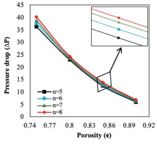
**Figure 21.** Variation of the pressure drop with porosity at Q=0.05046 lpm, phi-0.01.
