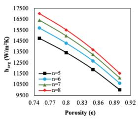
**Figure 11.** Variation of the average heat transfer coefficient with porosity at Q=0.05046 lpm, phi-0.01.
