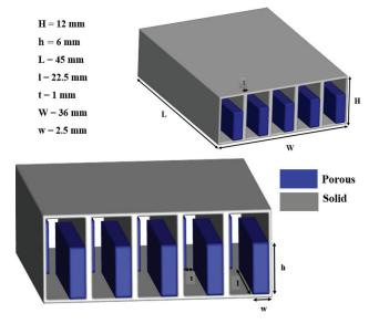
Figure 1. Schematic of the heat sink, including porous fins of Al-Cu3 foam.
