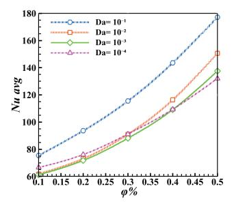
**Figure 13.** Nu<sub>avg</sub> as a function of nanoparticles concentrations  $\varphi$ % for various Da number at Re=3200, dn =20nm.
