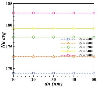
**Figure 14.** Changes of Nu<sub>avg</sub> with dn at different Re for  $\varphi = 0.5\%$ , Da=10<sup>-1</sup>.
