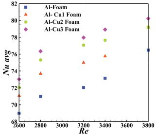
**Figure 6.** Average Nusselt number changes for various porous foams studied and Re number for  $\varphi$ =0.1%.
