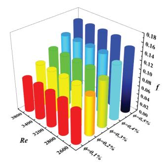
**Figure 18.** Friction factor as a function of Re at various concentrations of nanoparticles.
