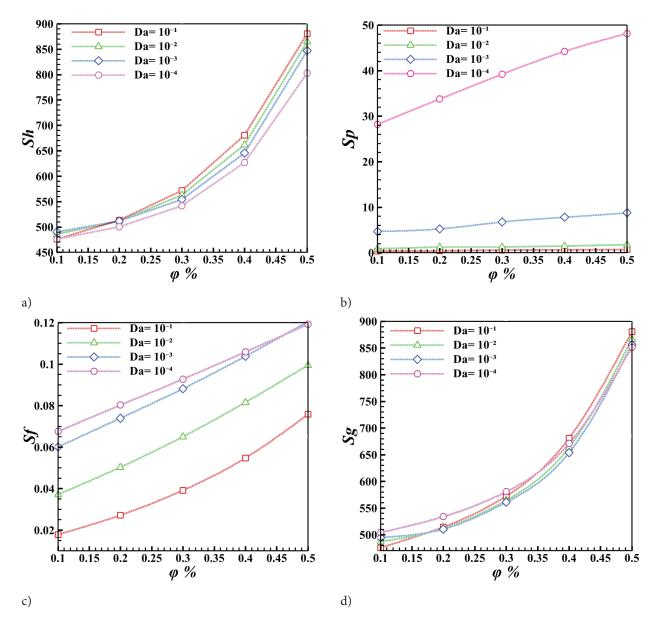
**Figure 16.** Changes of a)  $S_h$ , b)  $S_p$ , c)  $S_p$  and d)  $S_g$  with  $\varphi$ % at different Da for Re= 3200, dn =20nm.
