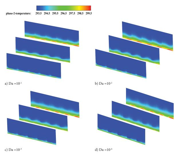
**Figure 10.** Heat sink temperature contours on the z-plane (5mm, 22.5mm, and 40mm) for various Da at Re =3200,  $\varphi = 0.3$ %, dn=20nm.
