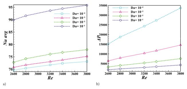
**Figure 12.** Variation of Nu<sub>avg</sub> and pressure drop in Re at different Da for  $\varphi = 0.2\%$ , dn=10nm.
