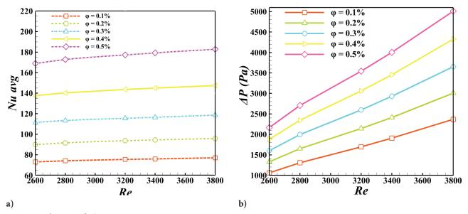
**Figure 8.** Changes of a) Nu<sub>avg</sub>, b)  $\Delta P$  with Re at different nanoparticle concentrations  $\varphi$  % for Da=10<sup>-1</sup>, dn=10 nm.
