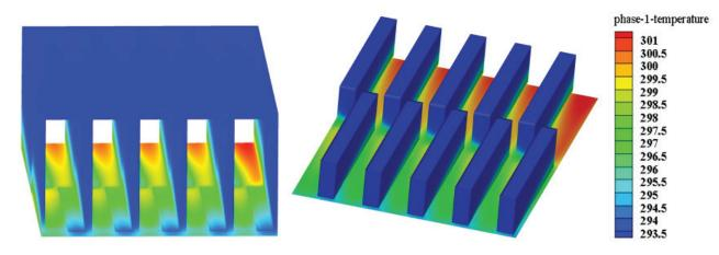
Figure 9. Effect of metal foam's position on temperature variation (K).
