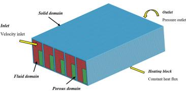
Figure 2. Mech topology and boundary conditions.
