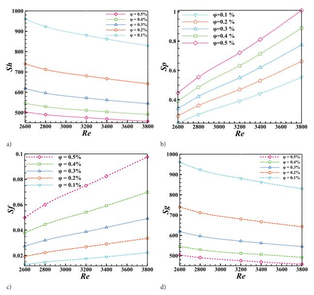
**Figure 15.** Effects of Re on entropy generation with different  $\varphi$ % at Da=10<sup>-1</sup>,dn =20nm.
