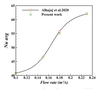
**Figure 4.** Comparison of  $Nu_{avg}$  of water in terms of different flow rates with the experimental results of Alhajaj et al. [50].
