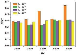
**Figure 19.** Performance evaluation criteria of HS with Da and Re numbers.
