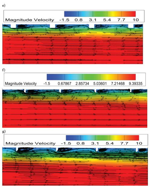
Figure 6. Velocity (m/s) profiles on different roughness elements.
