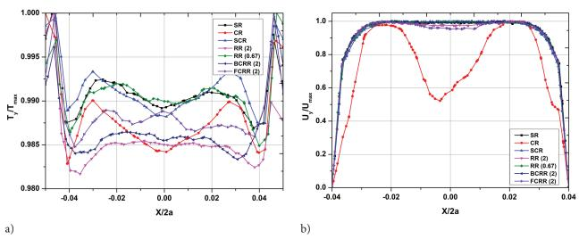
**Figure 10.** Changes in Temperature and Velocity Profiles at  $Z/I_{test}$ = 0.7 with Re of 20000 for different models.
