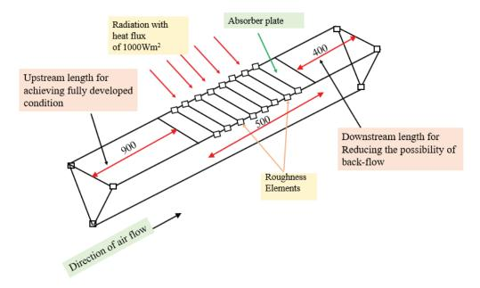
Figure 1. (a) Schematic Triangular SAH duct.
