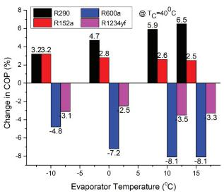
**Figure 10.** Change in COP (%) vs. Evaporator Temperature ( $Tc = 40^{\circ}C$ ).
