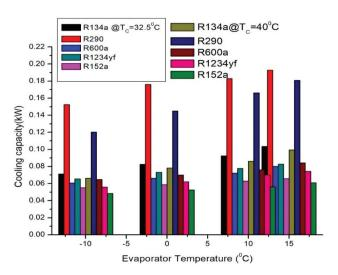
**Figure 3.** Cooling capacity vs. Evaporator temperature with LSHX.
