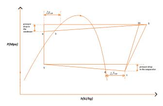
Figure 2. Pressure-enthalpy diagram.
