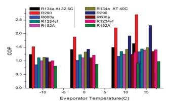
**Figure 8.** COP vs. Evaporator temperature without LSHX.
