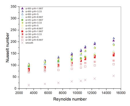
Figure 4. The Nu fluctuation in response to changes in Re, p/H, and angle of attack values.
