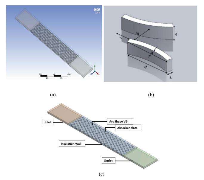
Figure 1. (a) The geometry in ANSYS design modeler (b) Schematic view of VGs arc staggered (c) Computational domain.
