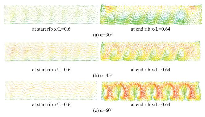
Figure 7. Velocity vector at YZ direction at Re=15000.
