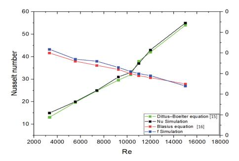
Figure 3. Validation of numerical results for flat plate SAH.
