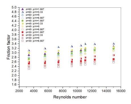
**Figure 11.** Variation of *f* ratio with Re at differed p/H and angle of attack.
