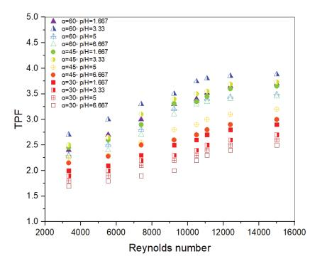
**Figure 12.** Changes in TPF as a function of Re at various p/H and attack angles.
