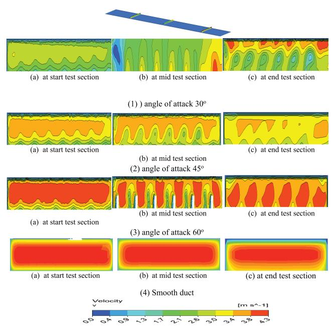
**Figure 8.** Contour of velocity profile at Re=15000 for (1) angle of attack 30° (2) angle of attack 45°(3) angle of attack 60° (4) Smooth duct.
