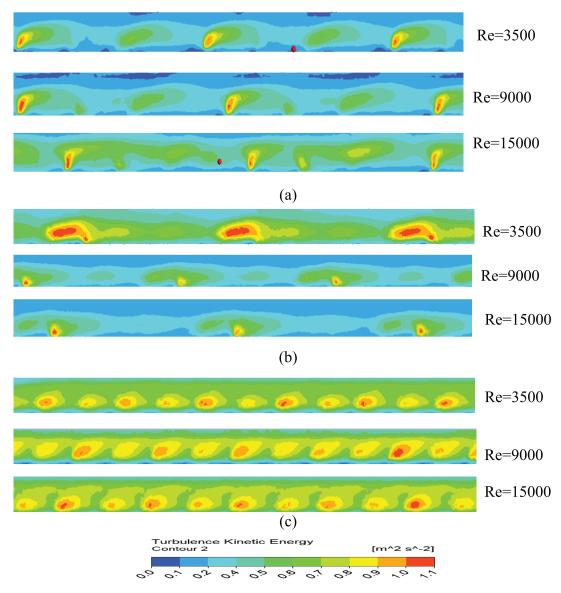
Figure 6. TKE contour for SAH at (a) angle of attack 30° (b) angle of attack 45° (c) angle of attack 60°.
