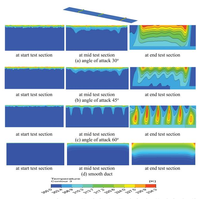
**Figure 9.** Temperature contour for Re15000 at (a) angle of attack 30° (b) angle of attack 45° (c) angle of attack 60° (d) Smooth duct.
