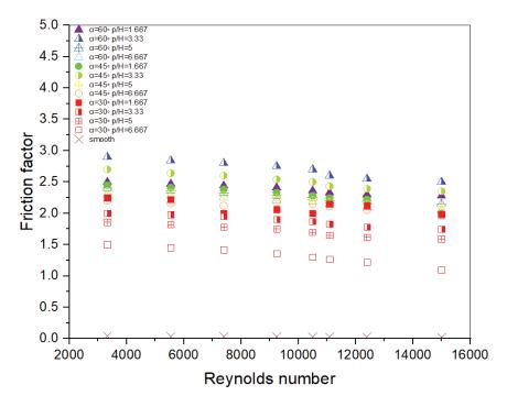
**Figure 10.** Changes in f as a function of Re at different p/H and attack angles.
