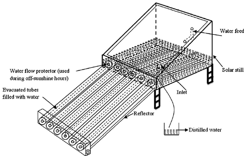
Figure 10. Schematic diagram for passive ETC solar still [From Singh et al. [57], with permission from Elsevier.]
