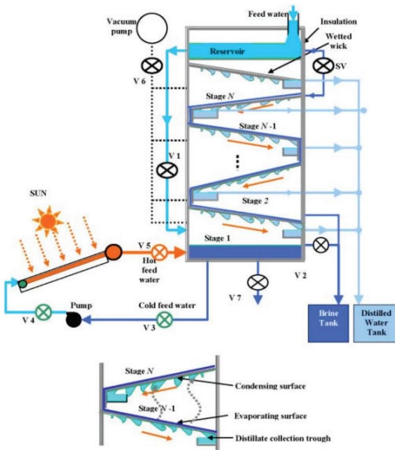
**Figure 5.** Flow inside solar distillation unit for active multistage series [From Reddy and Sharon [45], with permission from Elsevier.]
