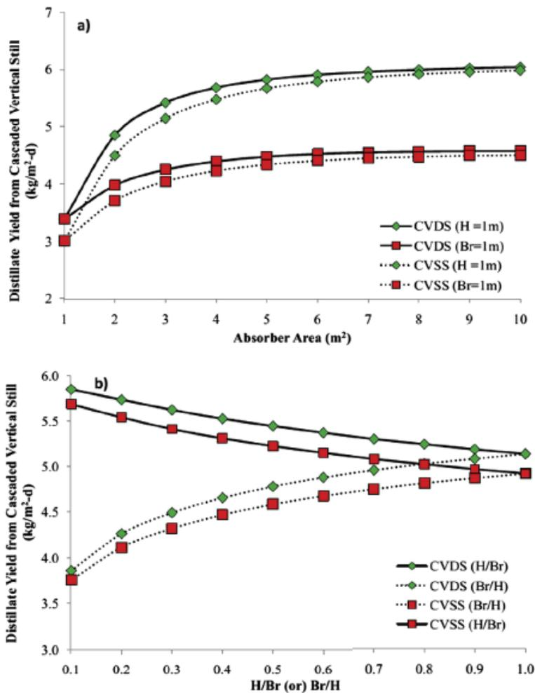
Figure 1. Impact of a) Area of absorber and b) Aspect ratio of cascaded vertical still on distillate yield [From Sharon and Reddy [37], with permission from Elsevier.]
