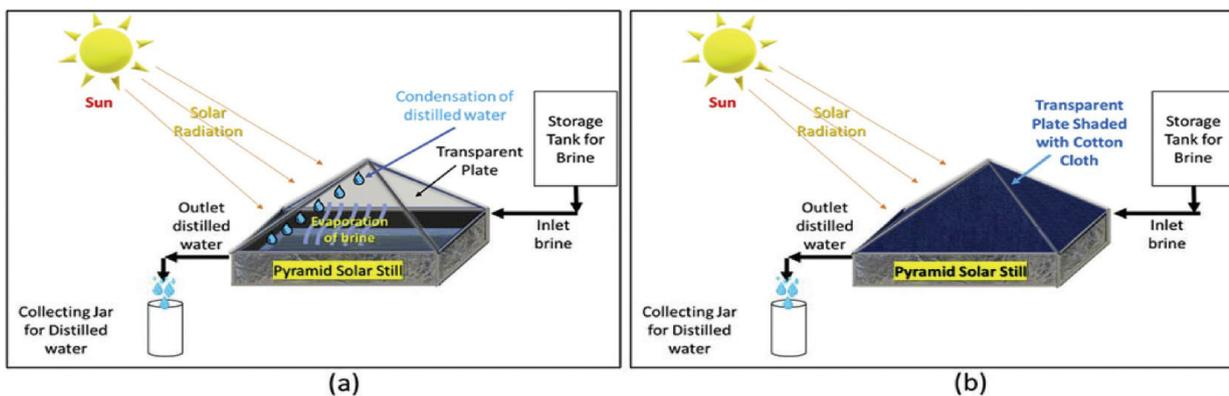
**Figure 6.** Schematic diagram of pyramid solar still CPS (a) without shading, (b) with shading SPS [From Kumar et al. [50], with permission from Elsevier.]
