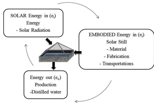
**Figure 7.** Simple cyclic flow chart of energy analysis for Pyramid shape still. S. [From Kumar et al. [50], with permission from Elsevier.]
