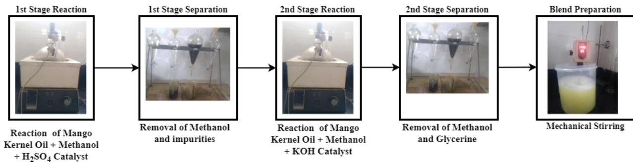
Figure 2. Biodiesel blend production process.
