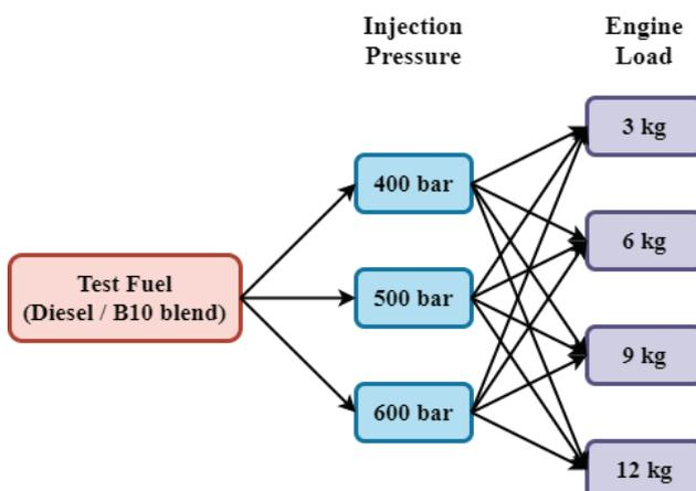
**Figure 4.** Network diagram for experimental tests.**Table 3.** Percentage uncertainty of measurement parameter
