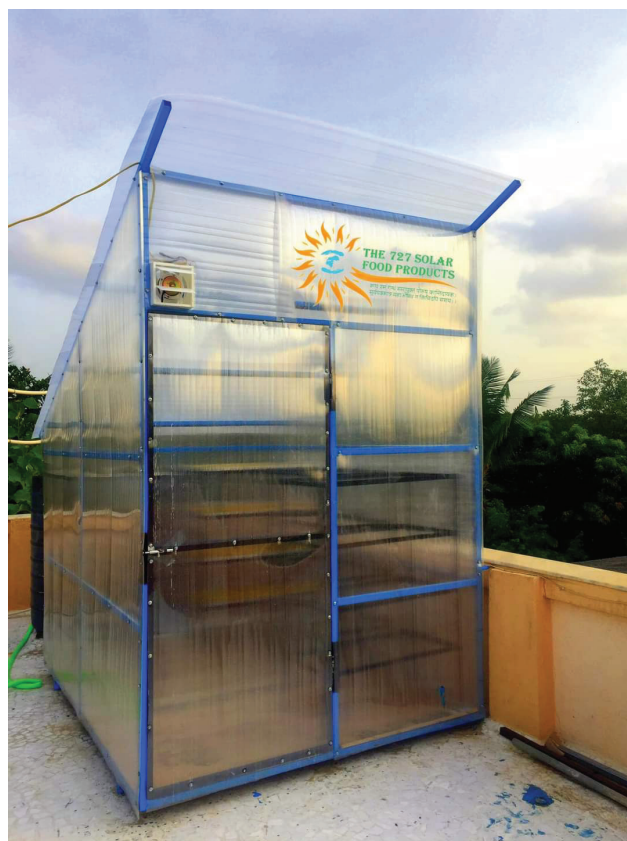
Figure 2. Experimental setup of greenhouse solar dryer.
