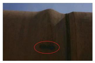
Figure 2. Deformation of the outer wall of the rotary cement kiln.
