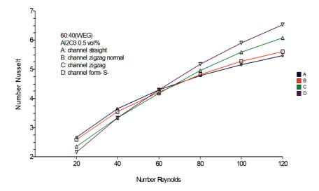
Figure 6. Nusselt number vs. Reynold number of the four models with nanofluid (Al<sub>2</sub>O<sub>3</sub>-W (60) / EG (40) mixture).
