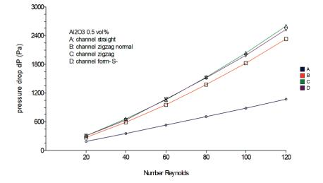
Figure 7. Pressure drop of the nanofluid (Al<sub>2</sub>O<sub>3</sub>-W mixture (60) / EG (40)) versus Reynolds number.
