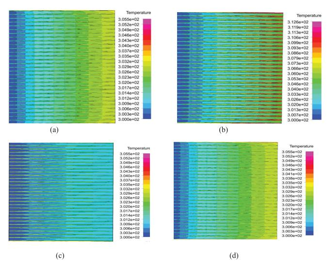
**Figure 13.** Temperature distribution of fluids in two stages straight plate for co- current and counter-current cases: a) First stage co-current, b) Second stage co-current, c) First stage counter-current, d) Second stage counter-current.
