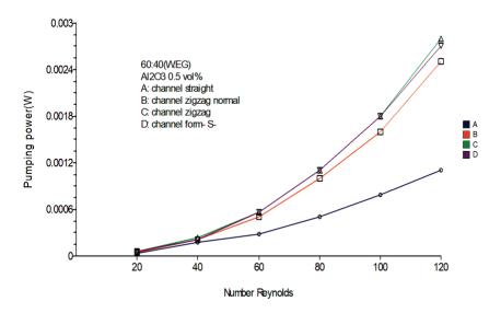
Figure 8. The pumping power of the nanofluid (Al<sub>2</sub>O<sub>3</sub>-W (60) / EG (40) mixture) versus Reynolds number.
