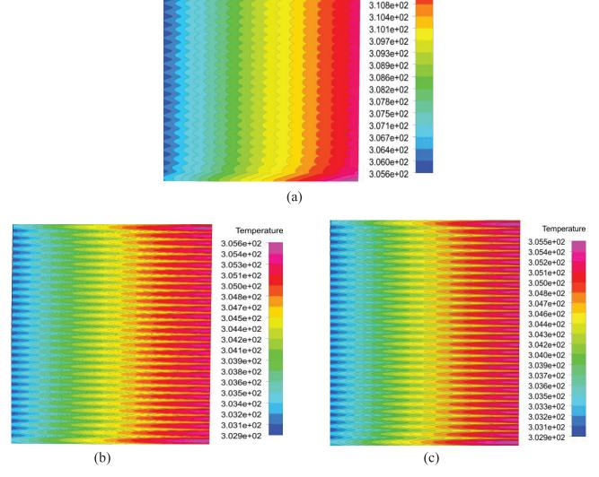
**Figure 12.** Temperature distribution at the area of wall for three straight plates: a) Straight plate simple, b) two stages Straight plate co- current and c) two stages Straight plate counter-current.
