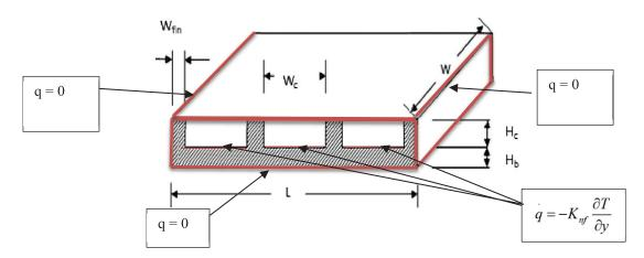
Figure 1. Schematic diagram of the microchannel in the PEMFC cooling plate.
