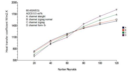
Figure 5. Heat transfer coefficient h for the four nanofluid models (Al<sub>2</sub>O<sub>3</sub>-W (60) / EG (40) mixture).
