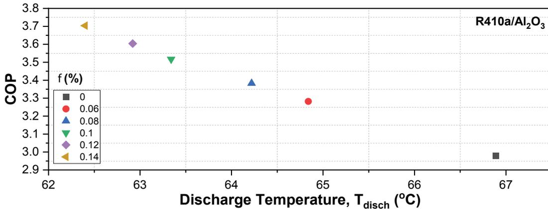
Figure 8 (c). COP of R410a/Al<sub>2</sub>O<sub>3</sub> as the function of discharge temperature.
