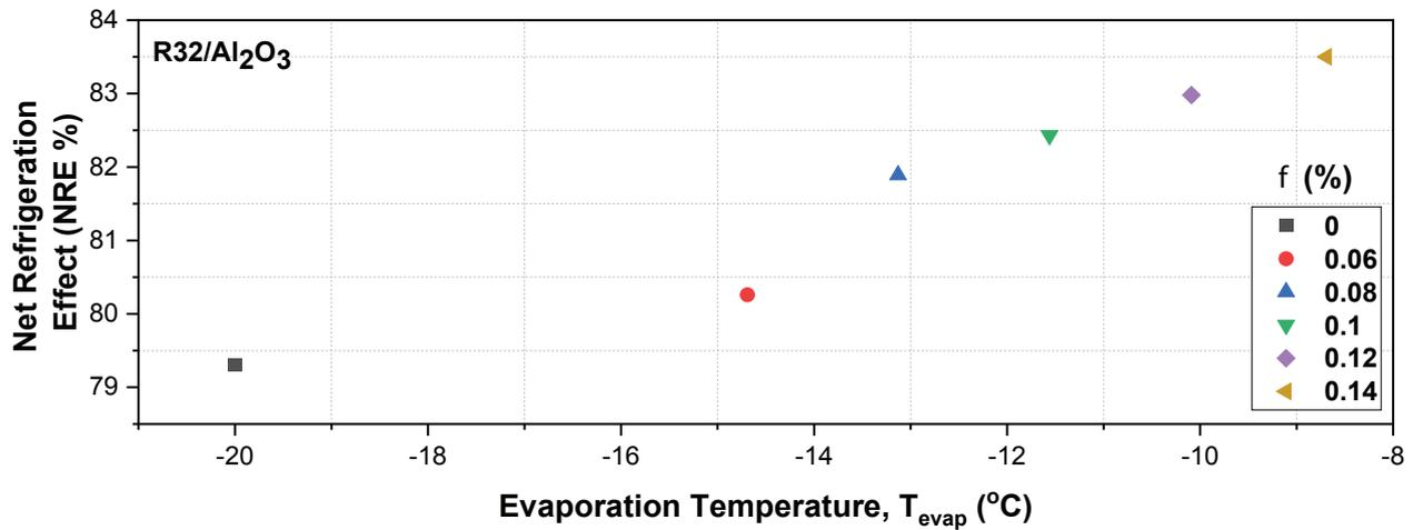
Figure 10 (b). Net refrigeration effect of R32/Al<sub>2</sub>O<sub>3</sub> as the function of evaporator temperature
