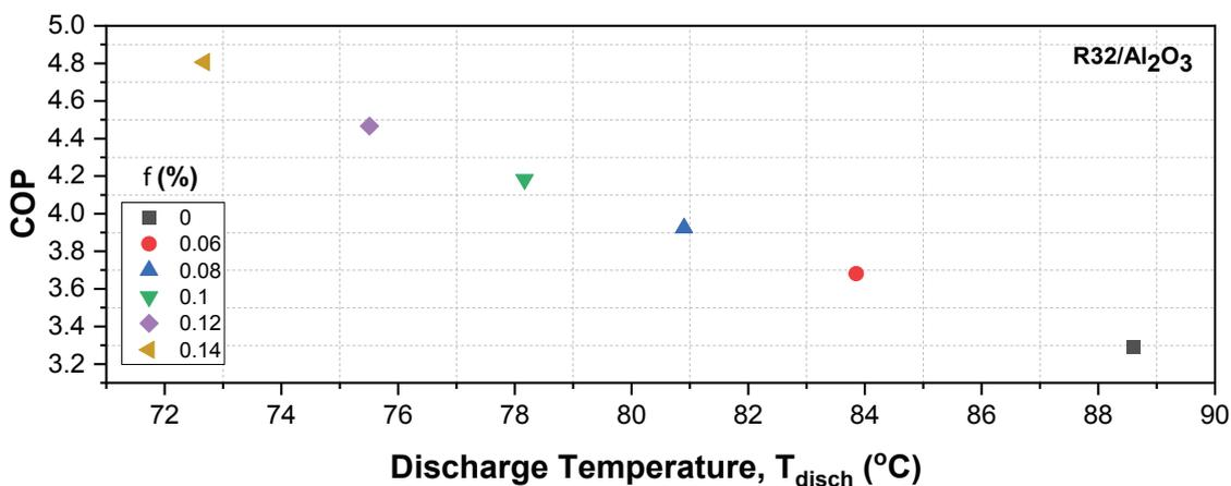
**Figure 8 (b).** COP of R32/Al<sub>2</sub>O<sub>3</sub> as the function of discharge temperature.
