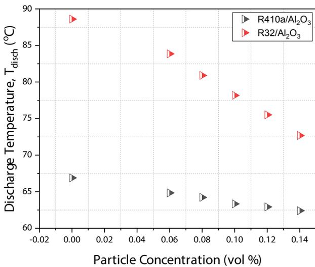
**Figure 8 (a).** Discharge temperature versus particle concentration.
