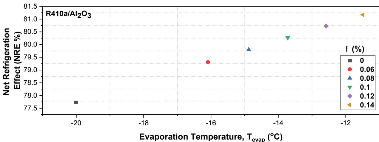
Figure 10 (a). Net refrigeration effect of R410a/Al<sub>2</sub>O<sub>3</sub> as the function of evaporator temperature
