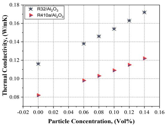
Figure 13. Increment of thermal conductivity of nanorefrigerants (R32/Al<sub>2</sub>O<sub>3</sub> and R410a/Al<sub>2</sub>O<sub>3</sub>) with the increase in particle concentration.
