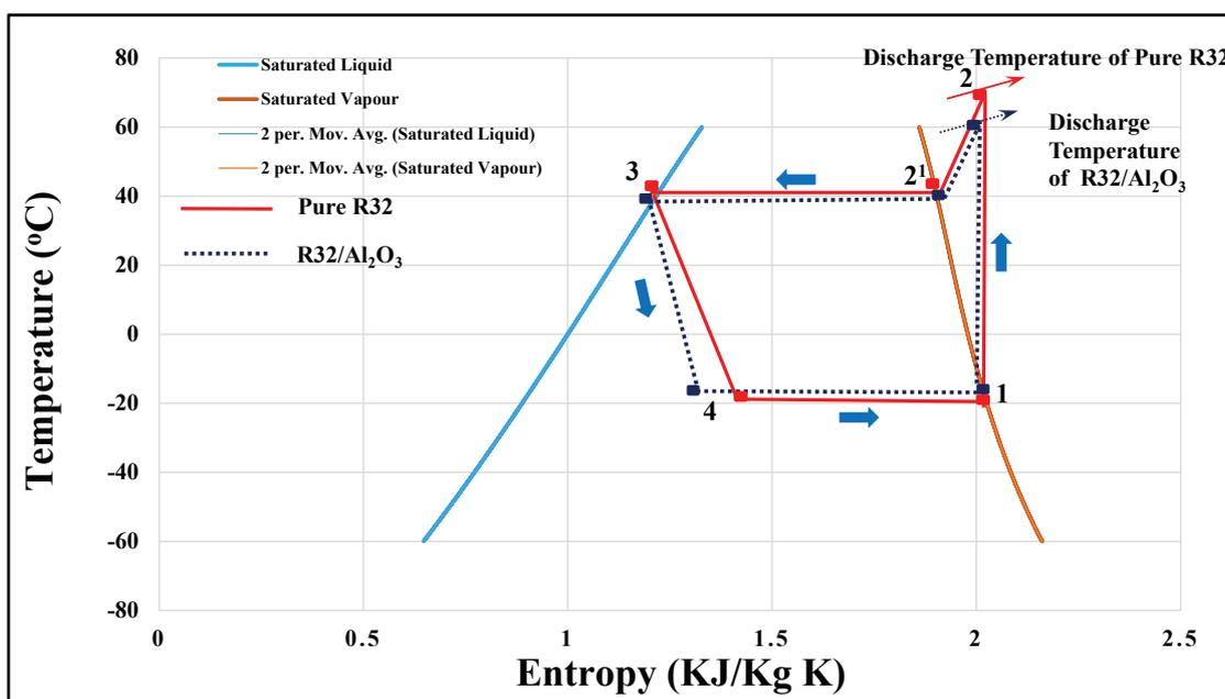
Figure 4. T-s diagram for pure and  $\text{Al}_2\text{O}_3$  nanorefrigerant cycle (R32).
