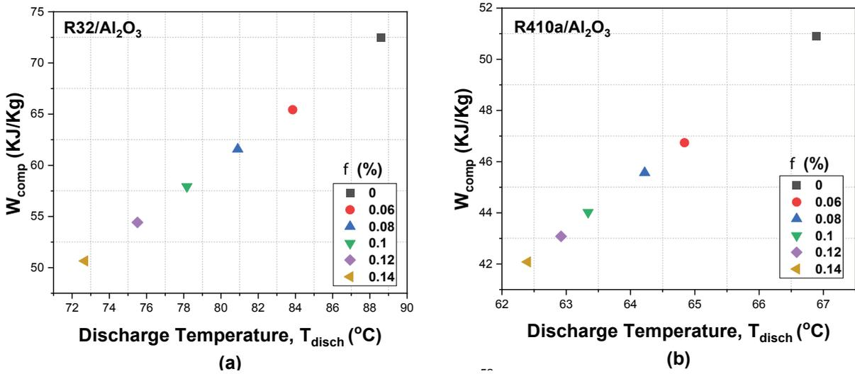
Figure 12 (a) and (b). Compressor work done versus discharge temperature.
