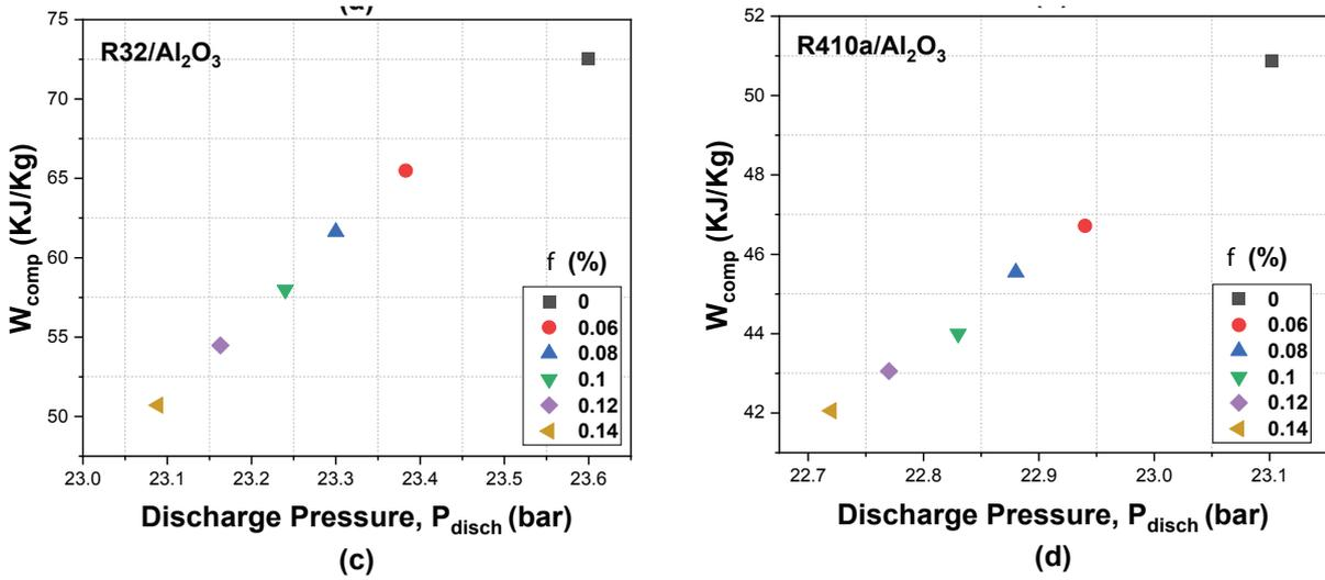
Figure 12 (c) and (d). Compressor work done versus discharge pressure
