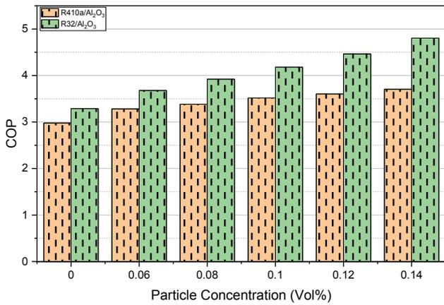
Figure 9. COP of the system as the function of various particle concentrations.
