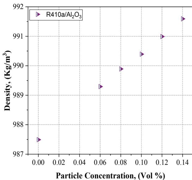
**Figure 15 (a).** Variation of density of R410a/Al<sub>2</sub>O<sub>3</sub> with particle volume concentrations.
