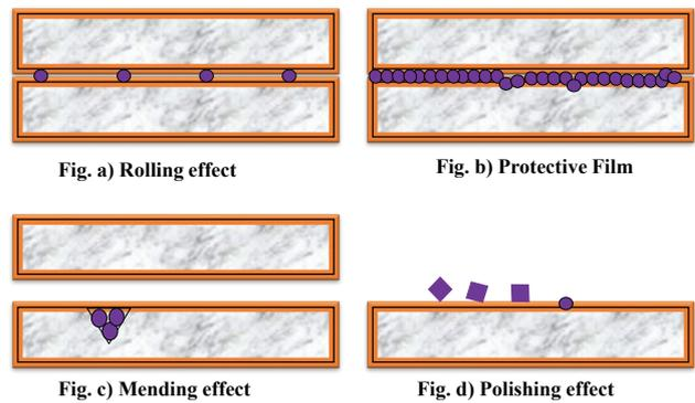
Figure 1. Lubrication mechanisms by the use of nanofluid in machining.
