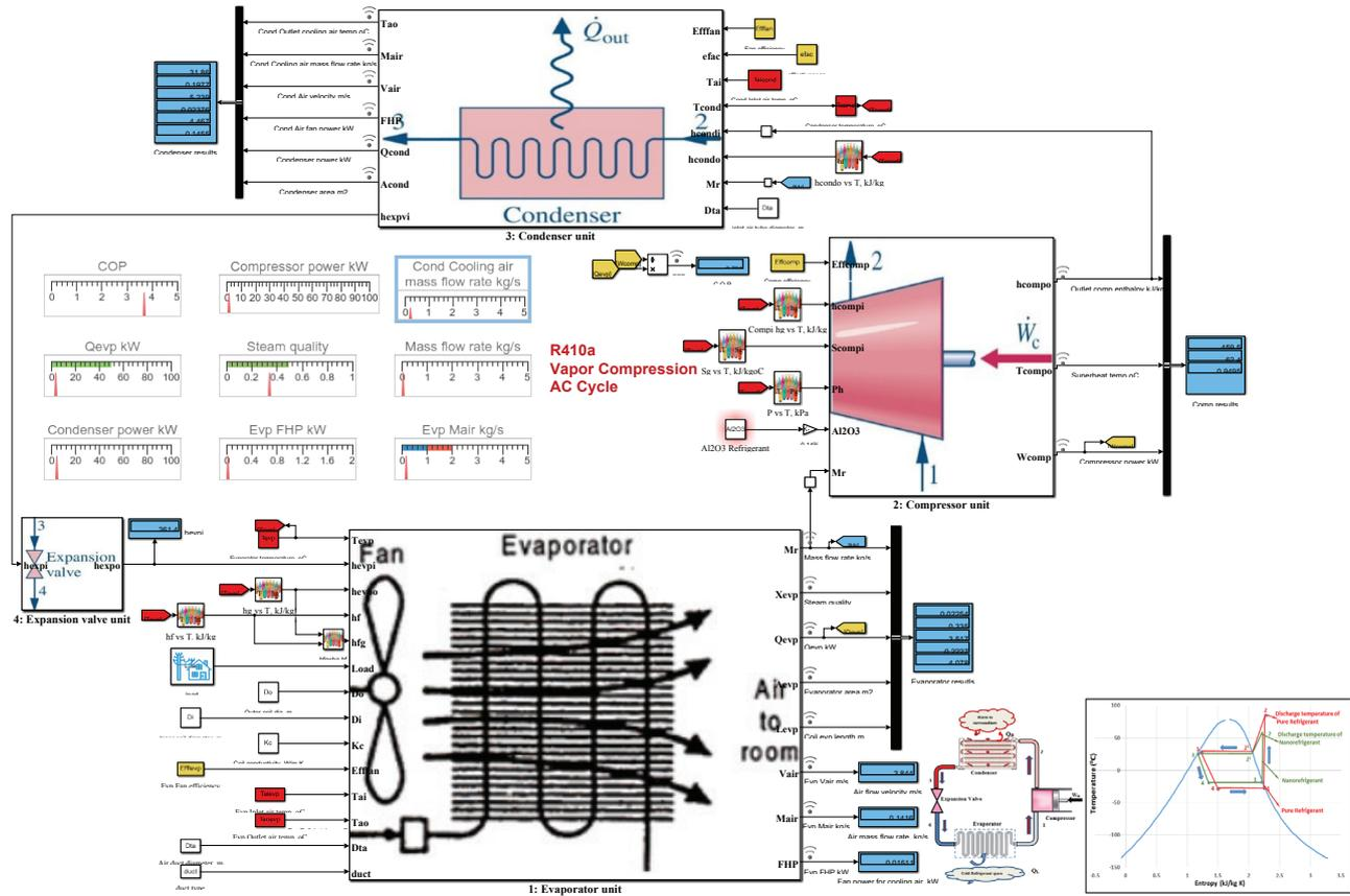
Figure 5 (b). Air Conditioning Framework used R410a/Al<sub>2</sub>O<sub>3</sub> Nanorefrigerant in Simulink.
