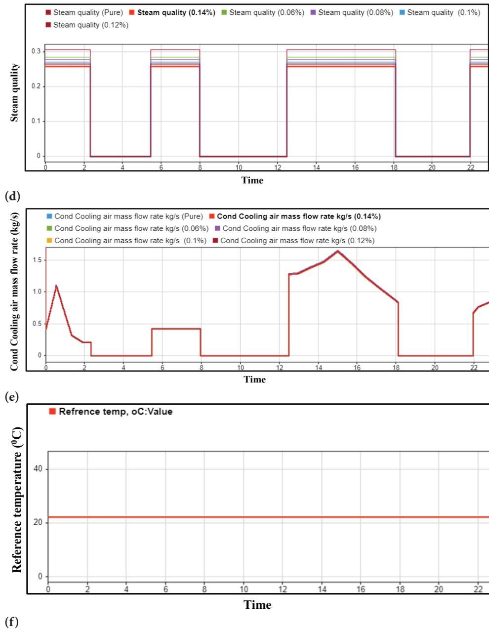
Figure 7. Performance of AC system with HFC-32/Al<sub>2</sub>O<sub>3</sub> nanorefrigerant according to cooling load with time response.
