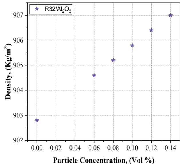
**Figure 15 (b).** Variation of density of R32/Al<sub>2</sub>O<sub>3</sub> with particle volume concentrations.
