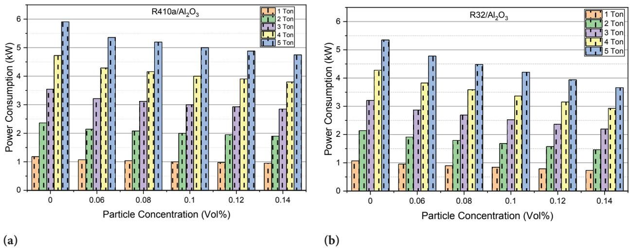
Figure 11. (a) and (b). Power Consumption vs Particle Concentration from 1 to 5 tons of refrigeration.
