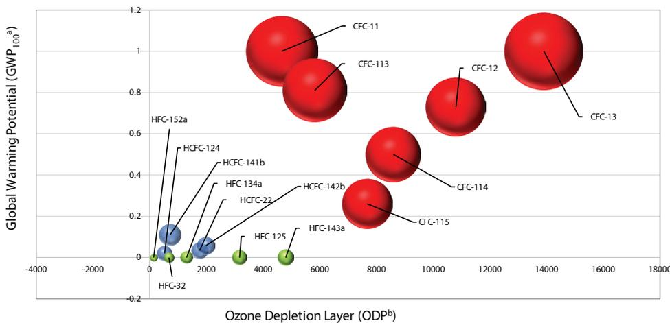
Figure 2. ODP versus GWP and lifetime of HFCs, HCFCs, CFCs (Circles).
