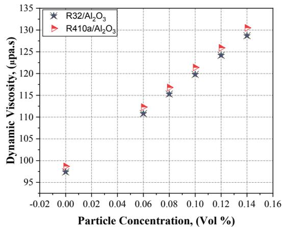
Figure 14. Variation of viscosity of (R32/Al<sub>2</sub>O<sub>3</sub> and R410a/Al<sub>2</sub>O<sub>3</sub>) with the increase in particle concentration.
