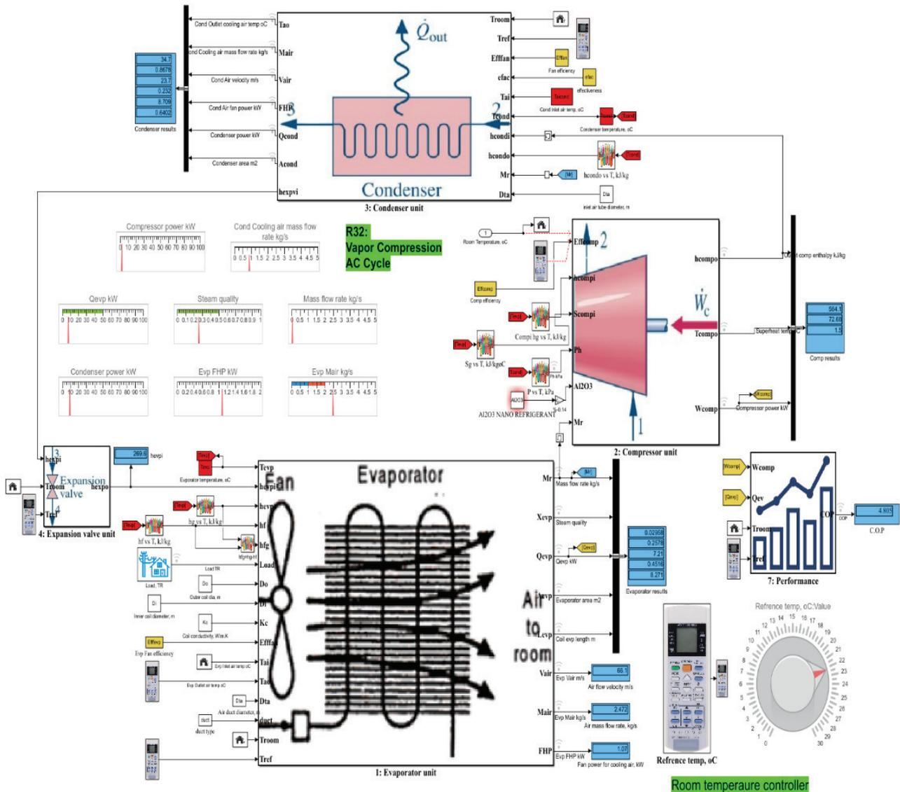
Figure 5 (a). Air Conditioning Framework used R32/Al<sub>2</sub>O<sub>3</sub> Nanorefrigerant in Simulink.
