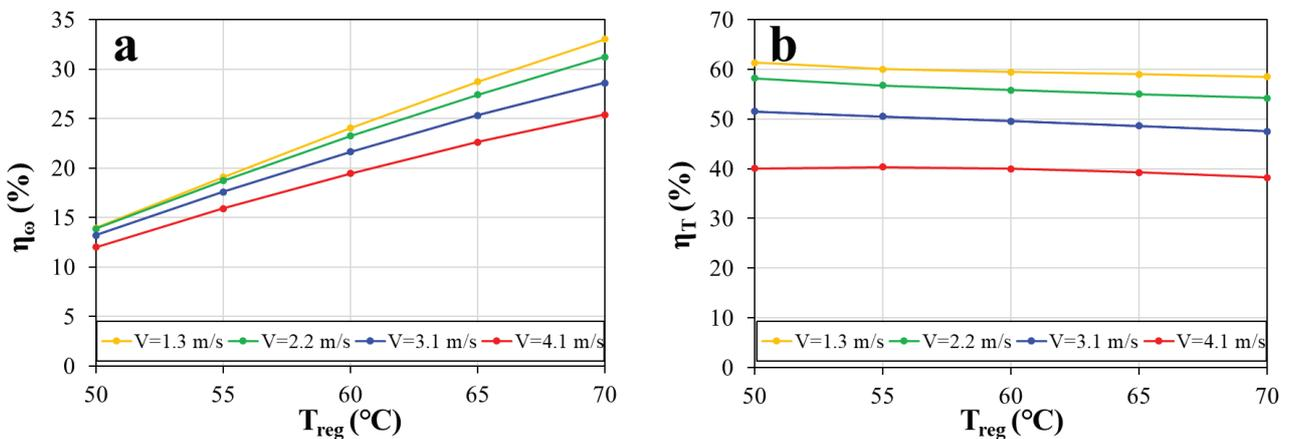
Figure 4. Dehumidification (a) and temperature effectiveness (b) of desiccant wheel.
