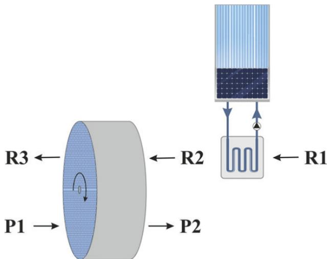
**Figure 1.** Schematic view of the desiccant wheel studied.
