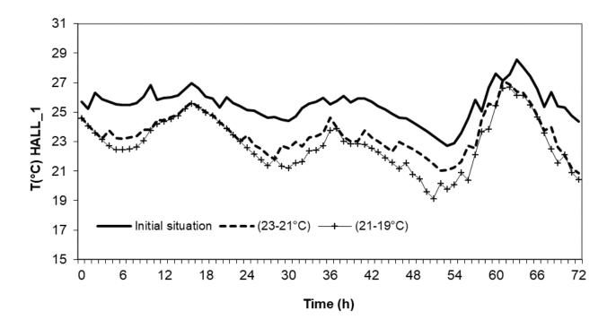
Figure 12. Effect of varying extraction threshold on the Hall\_1 temperature.
