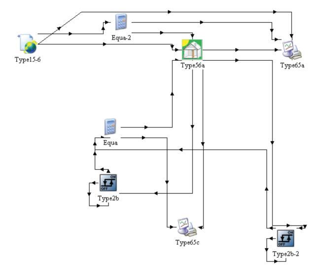
Figure 8. Schema of the TRNSYS system model.
