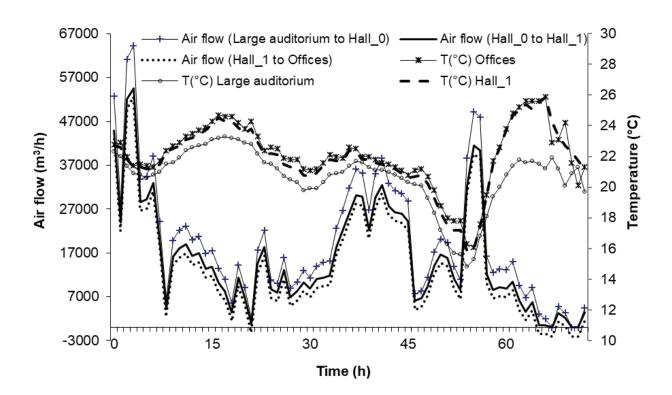
**Figure 18.** Temperatures and air flows values measured with natural ventilation circuit 2 (between large auditorium, Hall\_0, Hall\_1, and Offices), period of 23 to 26 July.
