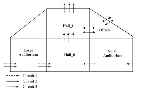
Figure 16. Natural ventilation circuits.
