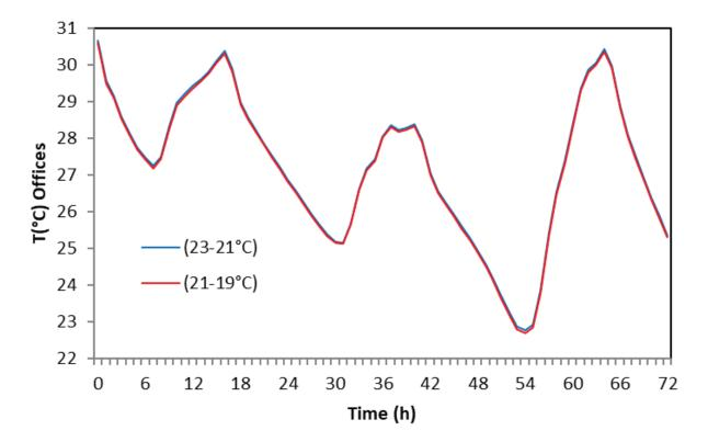
Figure 11. Effect of varying ventilation threshold on the offices' temperature.
