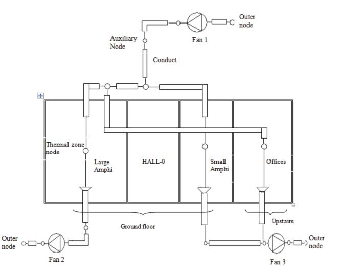
Figure 15. Simple model of the mechanical ventilation circuit that supplies the offices and the two auditoriums.
