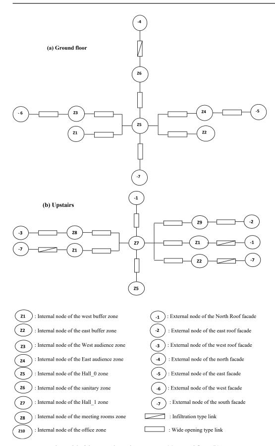
Figure 14. Simple model of the natural ventilation circuit, (a) ground floor, (b) upstairs.
