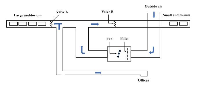
Figure 7. Diagram illustrating the direction of outdoor air conditioning in the building.
