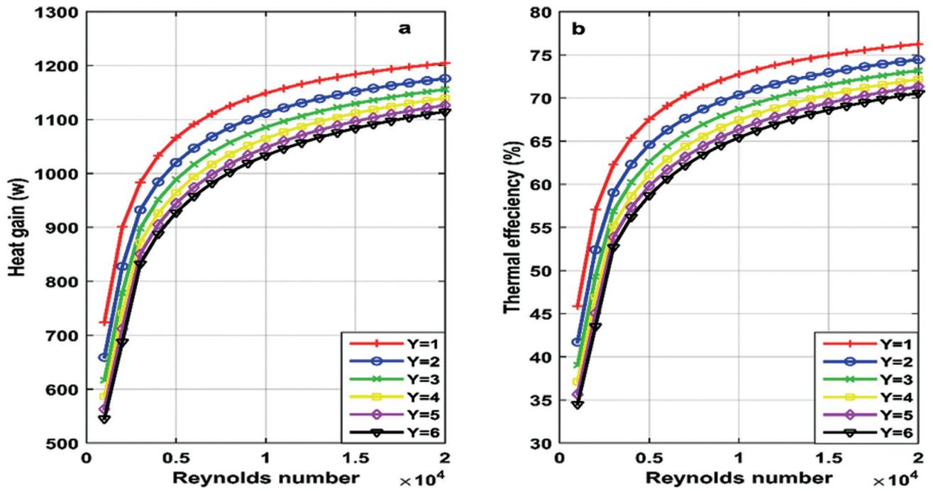
Figure 11. Influence of  $Y$  on the (a) heat gain, and (b) thermal efficiency.
