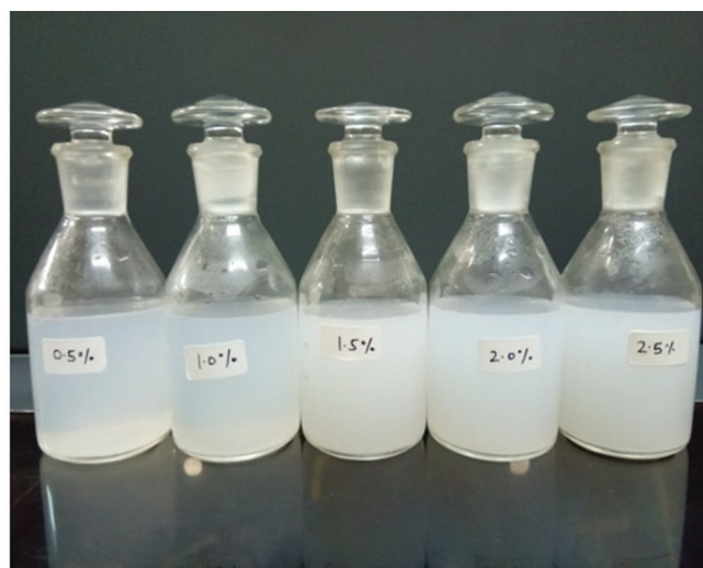
Figure 2. Sedimentation test for Al_2O_3 /H 2 O nanofluid, before and after 10 days.
