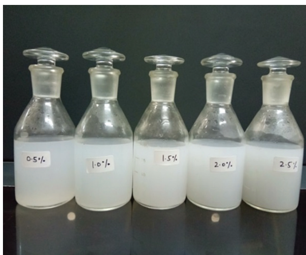
Figure 2. Sedimentation test for Al_2O_3 /H 2 O nanofluid, before and after 10 days.
