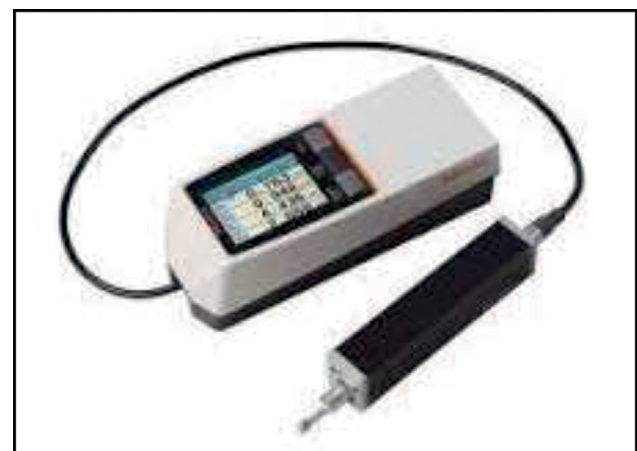
Figure 13. Profilometer used for surface roughness measurement.
