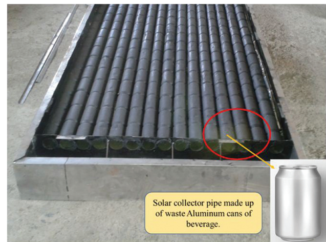
(B) Solar air collector made up of waste aluminum can.
