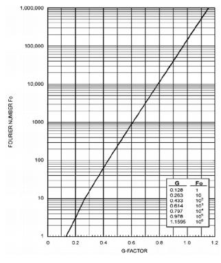
Figure 4. Relation between Fourier No. and G-Factor[14].
