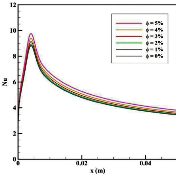
Figure 5. Distribution of local Nusselt along the heated wall at  $Re = 389$  with  $\phi = 0 - 5\%$ .
