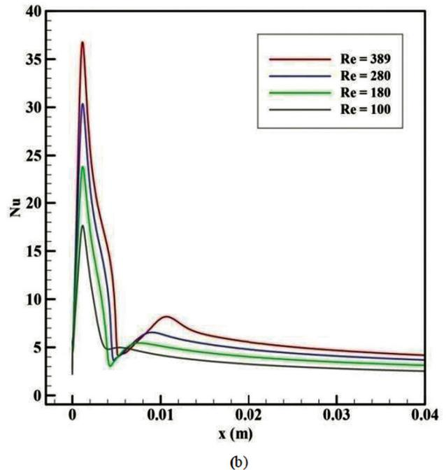
Figure 6. Effects of Reynolds number. (a) skin friction coefficient and (b) Nusselt number along the heated wall at  $Re = 100 - 389$  with  $\phi = 5\%$ ,  $H_b = 640 \mu m$  and  $D = 1$ .
