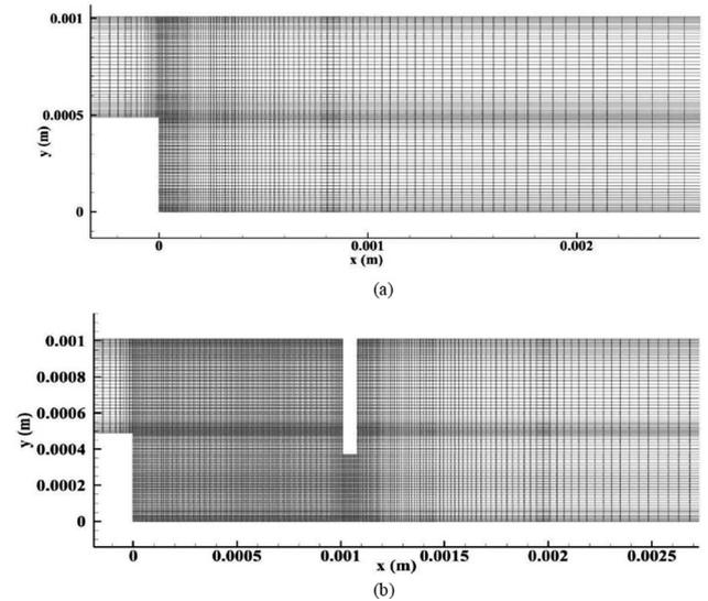
**Figure 2.** Grid structure. (a) without baffle and (b) with baffle.
