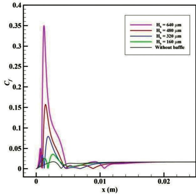
**Figure 10.** Distribution of local skin friction coefficient along the heated wall for  $Re = 389$  with increasing baffle height.
