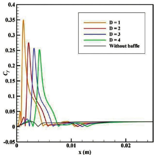
**Figure 13.** Effect of baffle distance on local skin friction coefficient at  $Re = 389$ ,  $\phi = 5\%$  and  $H_b = 640 \mu m$ .
