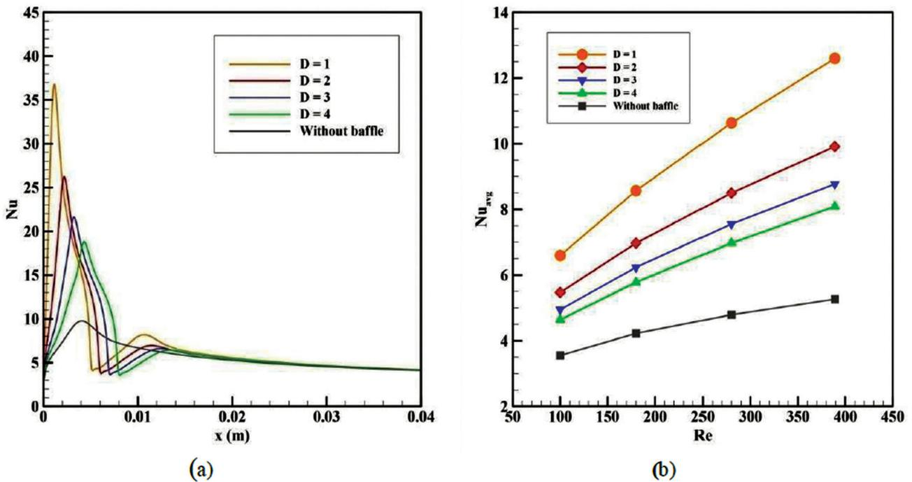
**Figure 12.** Effect of baffle distance. (a) local Nusselt number at  $Re = 389$ ,  $\phi = 5\%$ ,  $H_b = 640 \mu m$  and (b) average Nusselt number at  $Re = 100 - 389$ ,  $\phi = 5\%$  and  $H_b = 640 \mu m$ .
