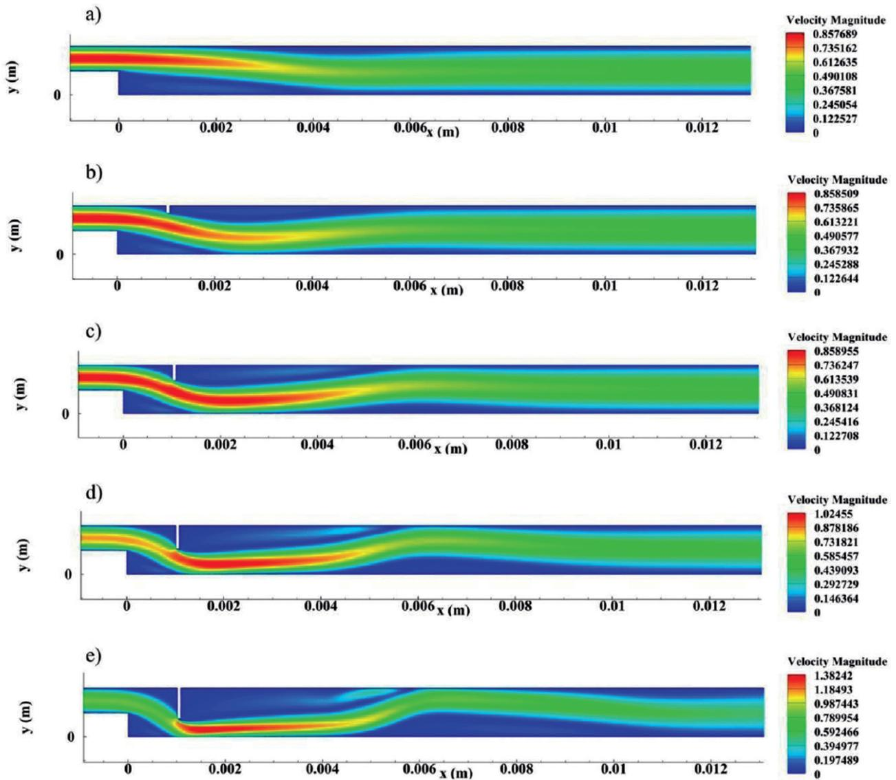
**Figure 7.** Effect of baffle height on velocity distribution. (a) no baffle, (b)  $H_b = 160 \mu\text{m}$ , (c)  $H_b = 320 \mu\text{m}$ , (d)  $H_b = 480 \mu\text{m}$  and (e)  $H_b = 640 \mu\text{m}$  at  $Re = 389$  with  $\phi = 5\%$ .
