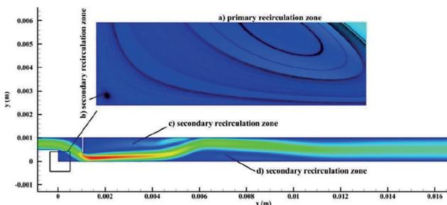
**Figure 8.** Flow structures. (a) primary recirculation zone near the step, (b) secondary recirculation zone near step corner, (c) secondary recirculation zone at the upper wall and (d) secondary recirculation zone downstream of the lower wall.
