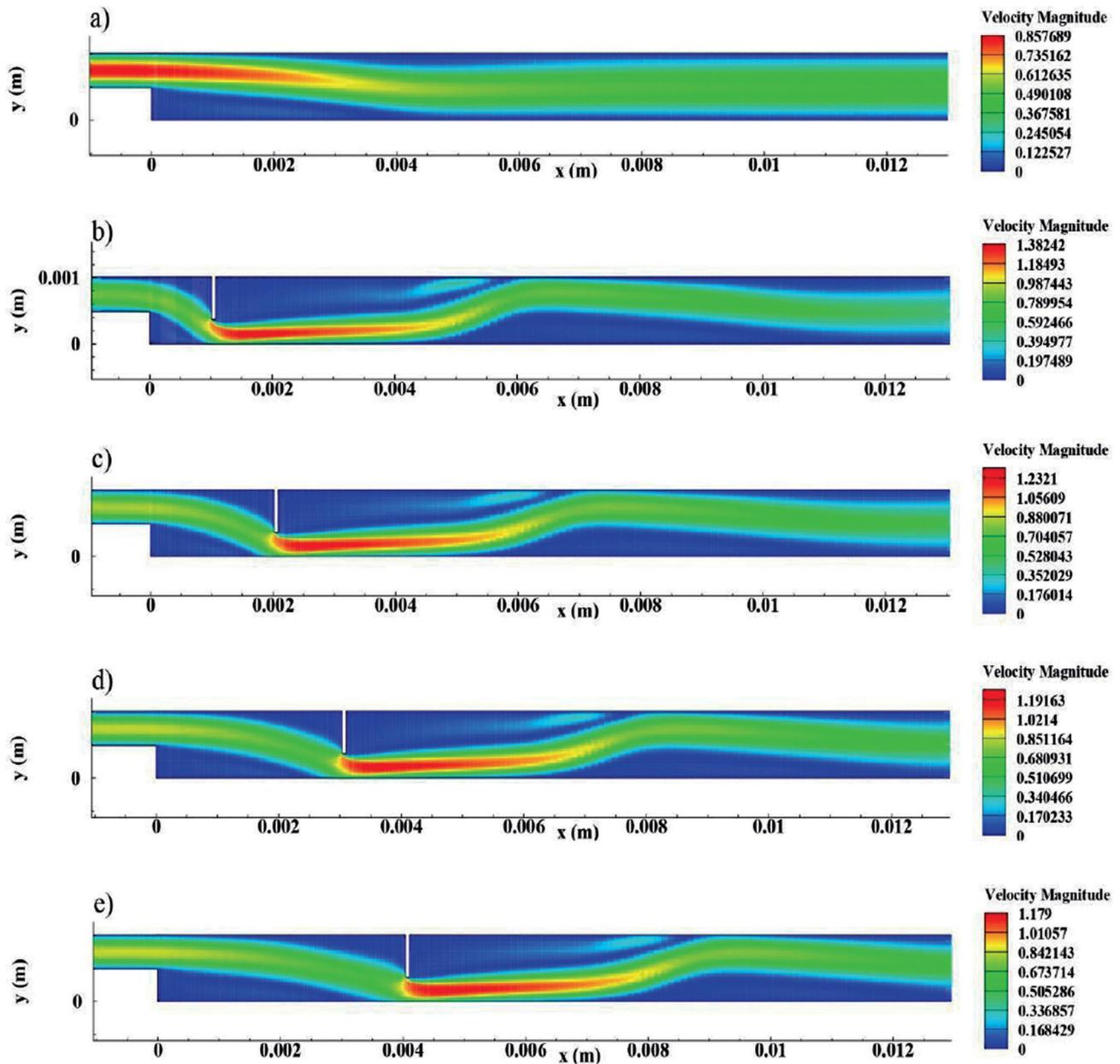
Figure 11. Contours of velocity. (a) no baffle, (b)  $D = 1$ , (c)  $D = 2$ , (d)  $D = 3$  and (e)  $D = 4$ .
