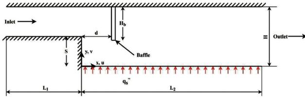
**Figure 1.** Computational model of micro-scale backward facing step channel with mounted baffle.
