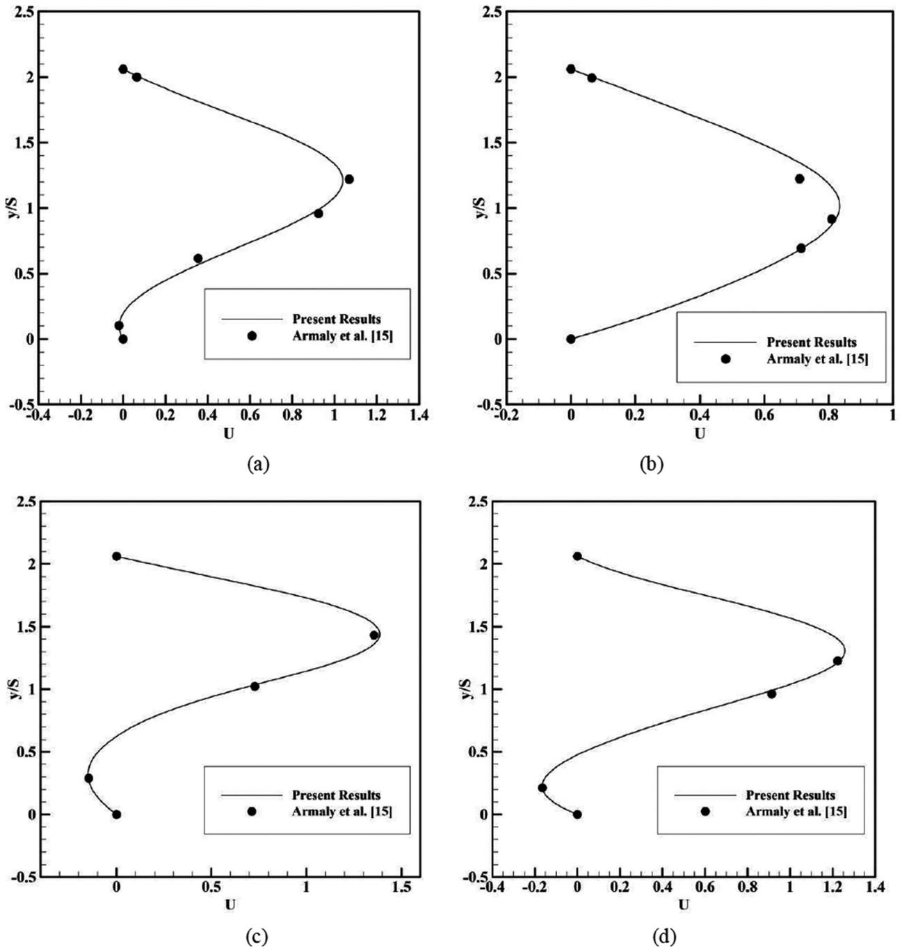
Figure 4. Comparison of the velocity distributions with the results of Armaly et al. [15]. (a)  $Re = 100$  at  $x/S = 2.55$ , (b)  $Re = 100$  at  $x/S = 4.8$ , (c)  $Re = 389$  at  $x/S = 2.55$  and (d)  $Re = 389$  at  $x/S = 4.8$ .
