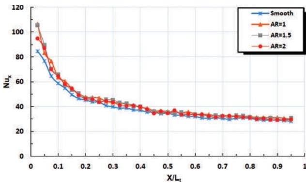
Figure 19. The effect of aspect ratio on local Nusselt number (BR=0.1, VGs=2).
