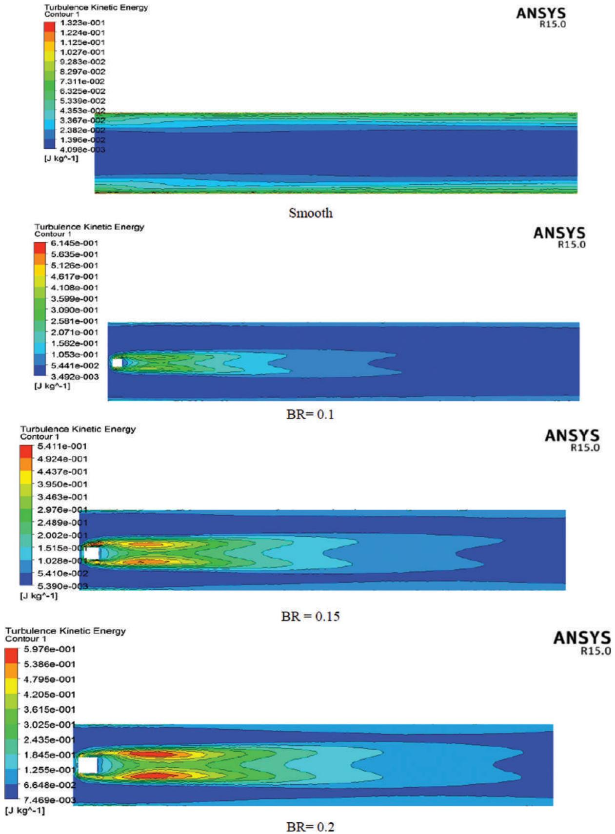
Figure 8. The contours of turbulence kinetic energy for different blocking ratio (BR).
