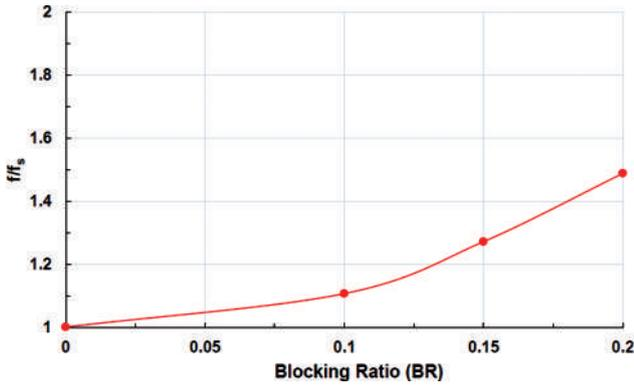
Figure 9. Variation of friction factor with blocking ratio.
