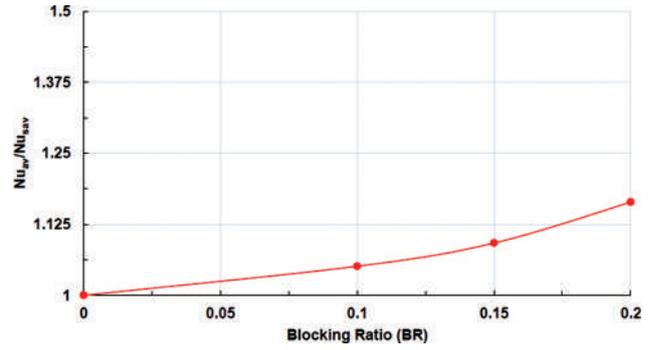
Figure 10. The variation of enhancement of average Nusselt number with blocking ratio.
