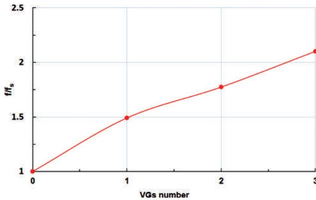
Figure 13. The variation of friction factor with VGs number (BR = 0.2).
