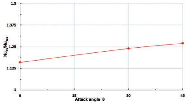
Figure 18. The variation of enhancement of average Nusselt number with attack angle (BR = 0.2, VGs = 3).
