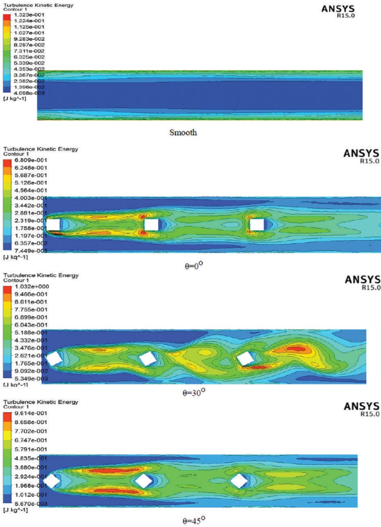
Figure 16. The contours of turbulence kinetic energy (BR=0.2, VGs=3).
