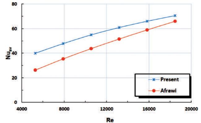
Figure 6. comparison of the present CFD prediction with experimental data from Afrawi [12].
