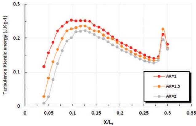
**Figure 22.** The variation of turbulence kinetic energy with Aspect ratio (BR = 0.1 , VGs=2).
