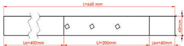
Figure 1. Side view of 3-D computational domain.
