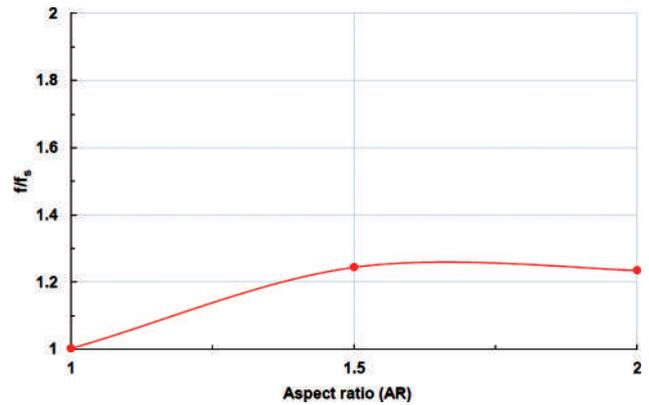
**Figure 23.** The effect of VGs aspect ratio on the friction factor (BR = 0.1, VGs = 2).
