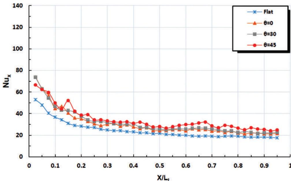
Figure 15. The variation of local Nusselt number with attack angle ( $V = 2$  m/s, BR = 0.2, VGs = 3).
