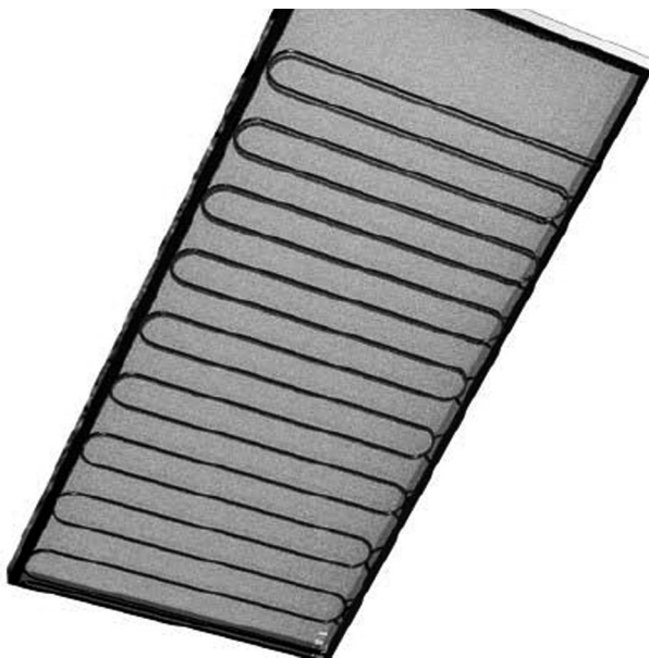
Figure 2. CAD model of the thermal collector.
